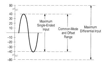
Figure 8: Input and Offset Range for X 0.1 Gain
