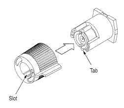
Figure 18: Replacing the TEKPROBE collar
