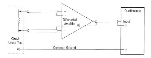
Figure 7: Eliminating Ground Loops in a Differential Setup
