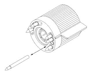
Figure 17: Replacing TEKPROBE Interface Pins
