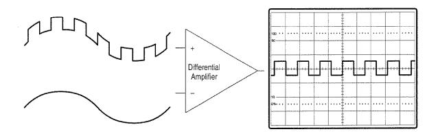
Figure 6: Differential Rejection of Common-Mode Signal
