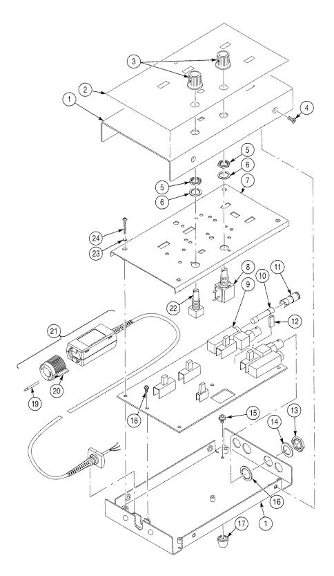
Figure 22: ADA400A Differential Preamplifier — Exploded View
