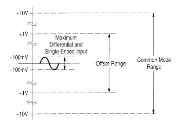
Figure 11: Input and Offset Range for X 100 Gain
