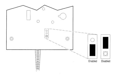
Figure 1: Configuration Jumper for Scale Factor Coding
