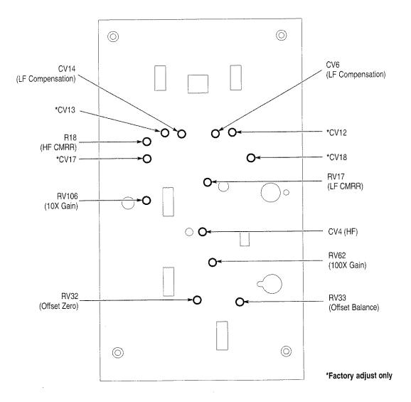
Figure 16: Location of Adjustments Underneath Inner Shield
