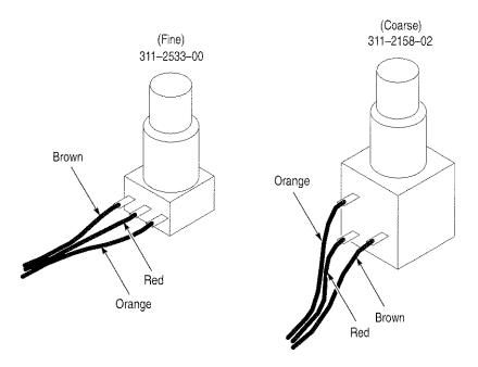
**Figure 20: Potentiometer Connections**
