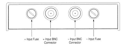
Figure 3: Input Connectors and Fuses
