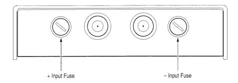
Figure 19: Input Connectors and Fuses
