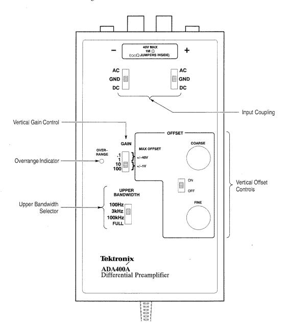
**Figure 2: Front Panel Controls**
