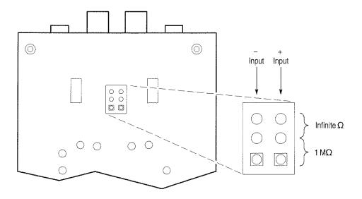
Figure 5: Selecting the Input Impedance
