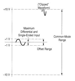
Figure 10: Input and Offset Range for X 10 Gain
