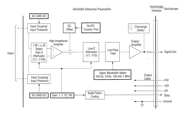
Figure 21: Diagram of the ADA400A Differential Preamplifier
