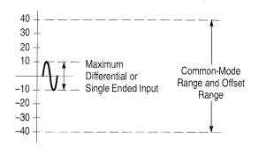
Figure 9: Input and Offset Range for X 1 Gain
