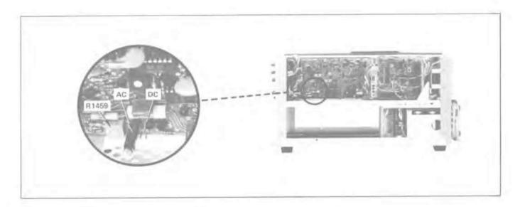
Figure 5-2. Location of Calibrator AC/DC jumper.
