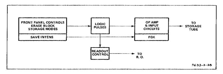
Figure 3-38. Storage circuit simplified block diagram.
