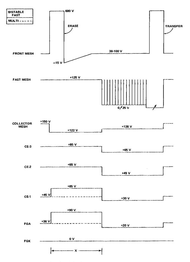
Figure 3-42. FAST BISTABLE mode Storage waveforms.
