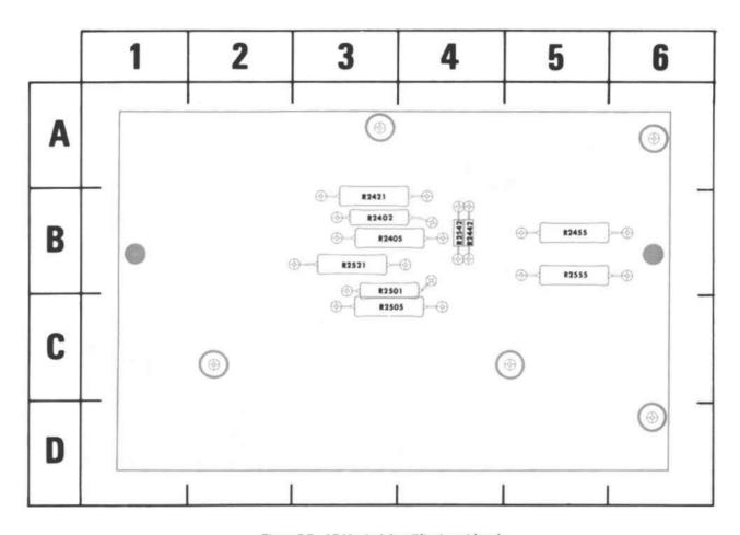
Figure 8-7. A5-Vertical Amplifier board (rear).
