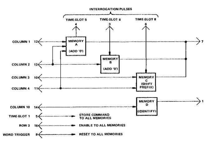
Figure 3-34. Block representation of memory sequence in U2232.
