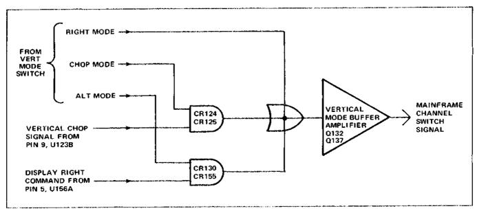
Figure 3-9. Logic diagram of Vertical Mode Control and Vertical Mode Buffer Amplifier stages.
