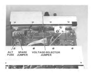
Figure 1-1. Location of voltage-selector jumper.
