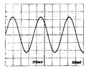
Figure 3-26. Typical readout display where only channel 2 of the Right Vertical and Horizontal units is displayed.
