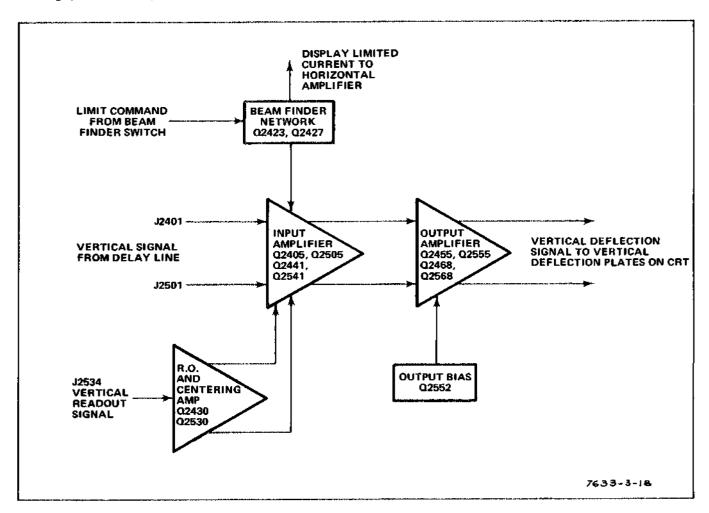
Figure 3-18. Vertical Amplifier detailed block diagram.
