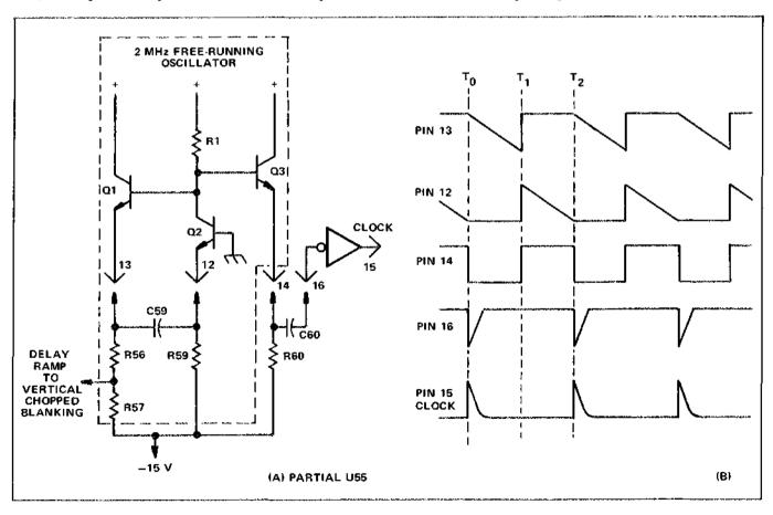
Figure 3-4. (A) Clock Generator stage of U55A. (B) Idealized waveforms from Clock Generator stage.
