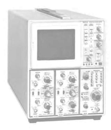
The Tektronix 7623A/R7623A Storage Oscilloscope is a solid-state instrument designed for fast writing rate storage applications. The 7623A operates in three display modes—NON STORE, STORE, and SAVE, and has four storage modes—BISTABLE, VAR PERSIST, FAST BISTABLE, and FAST VAR PERSIST. This instrument has three plug-in compartments that accept any 7-series plug-in units to form a highly flexible measurement system.
