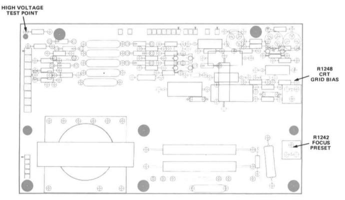
Figure 8-19. High Voltage board.
