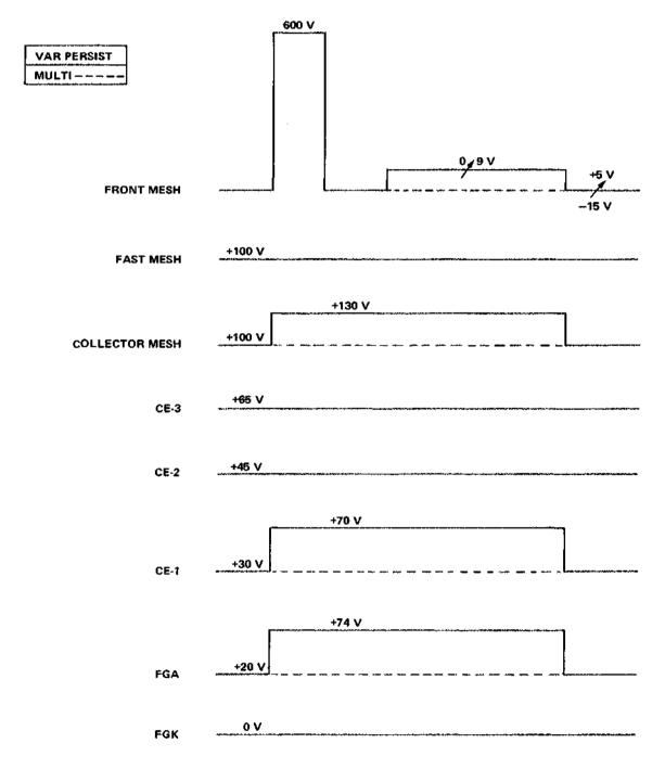
Figure 3-41. VAR PERSIST mode Storage waveforms.
