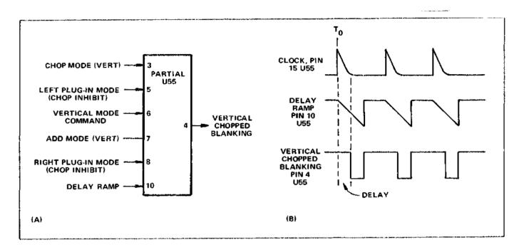
Figure 3-5. (A) Input and output pins for Vertical Chopped Blanking stage. (B) Idealized waveforms for Vertical Chopped Blanking stage.
