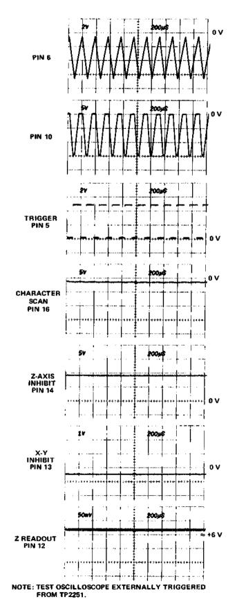
Figure 3-30. Timer stage operation when Display-Skip condition occurs.
