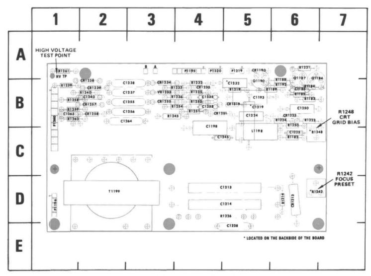
Figure 8-12. A10-High Voltage board.
