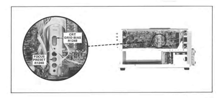
Figure 5-4. Location of adjustments in High-Voltage cover.
