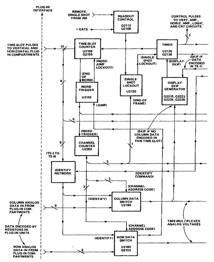
Figure 3-27. Detailed block diagram of the Reedout System.
