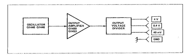
Figure 3-23. Calibrator detailed block diagram.
