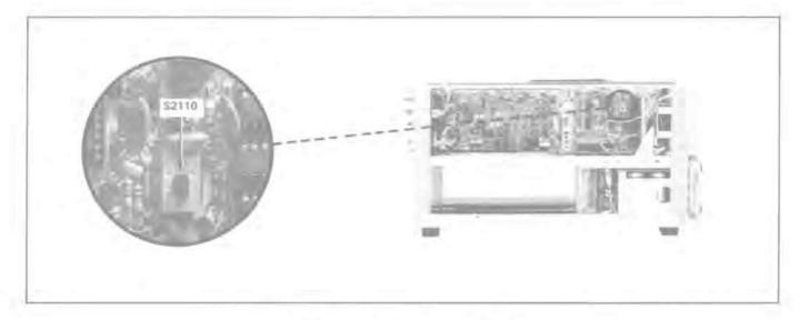
Figure 1-5. Location of Readout Mode switch.
