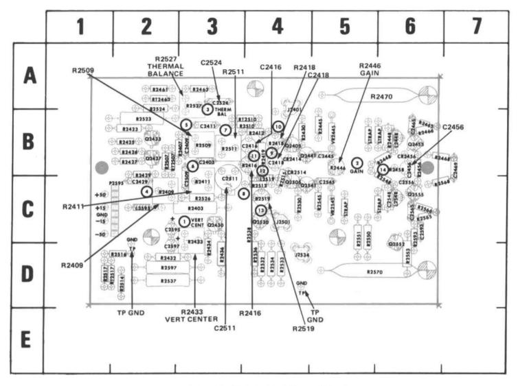
Figure 8-6. A5-Vertical Amplifier board (front).
