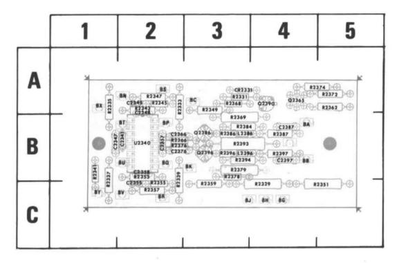
Figure 8-5. A4-Vertical Interface board.
