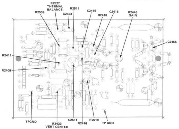
Figure 8-20. Vertical Amplifier board.
