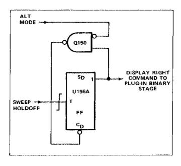
Figure 3-10. Logic diagram of Vertical Binary stage.
