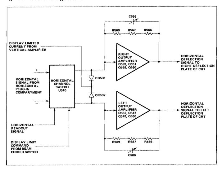
Figure 3-19. Horizontal Amplifier detailed block diagram.
