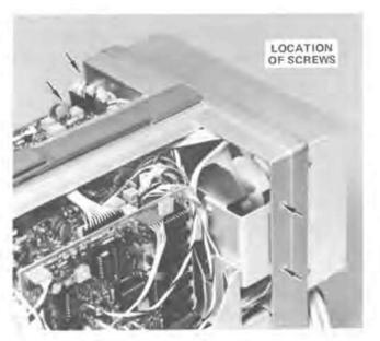
Figure 4-5. Location of screws holding Low-Voltage sub-chassis.
