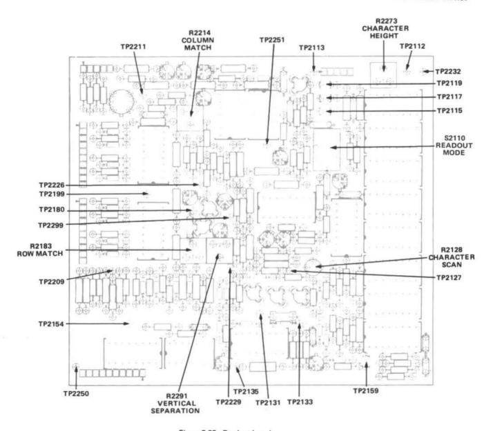
Figure 8-23. Readout board.
