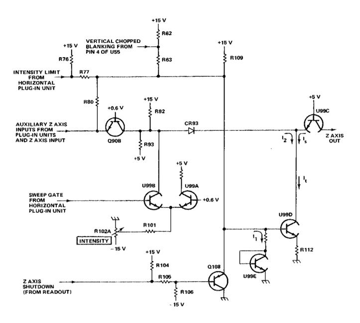
Figure 3-3. Z-Axis Logic block diagram.
