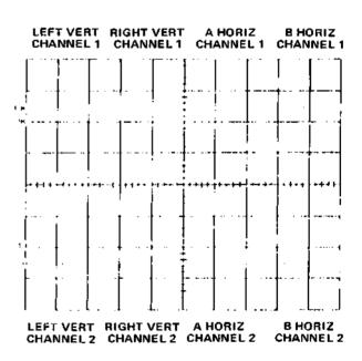
Figure 3-24. Location of readout words on the crt identifying the originating plug-in unit and channel (one complete frame shown).
