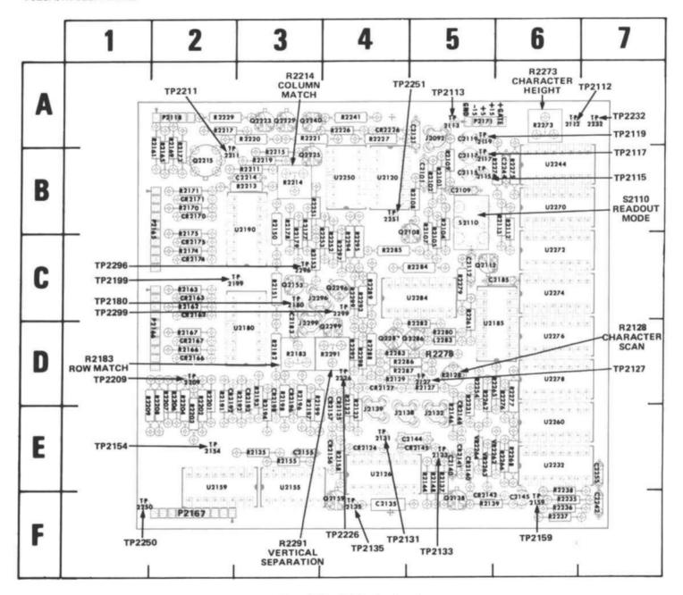
Figure 8-15. A13-Readout board.
