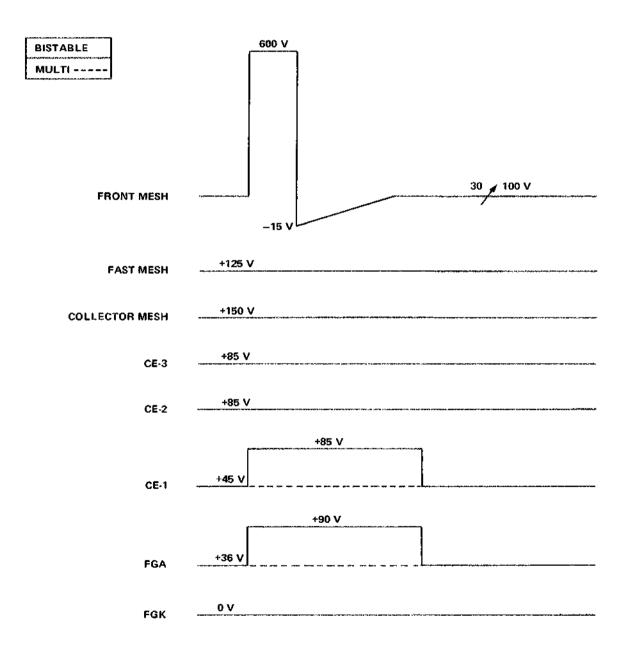
Figure 3-40. BISTABLE mode Storage waveforms.
