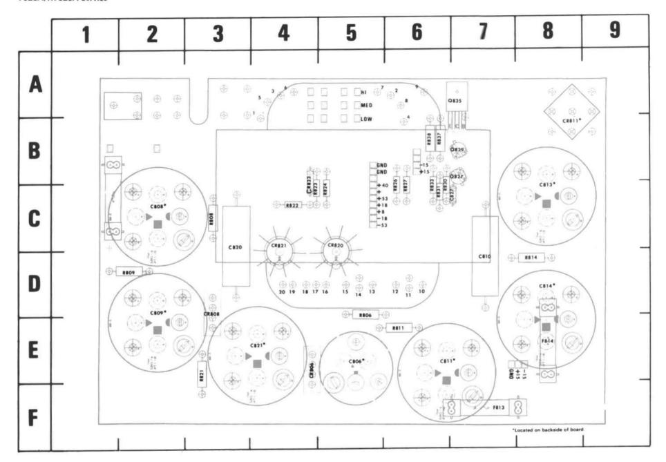
Figure 8-13. A11-Low-Voltage Rectifier board.
