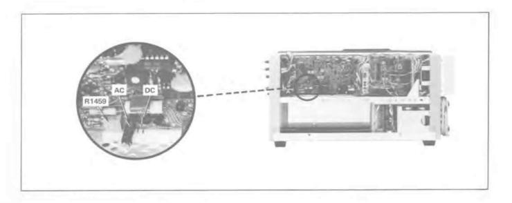
Figure 5-6. Location of Calibrator AC/DC jumper.
