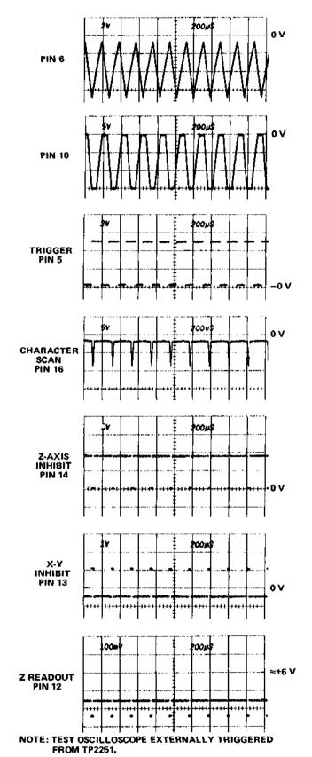
Figure 3-28. Output waveforms of Timer stage.
