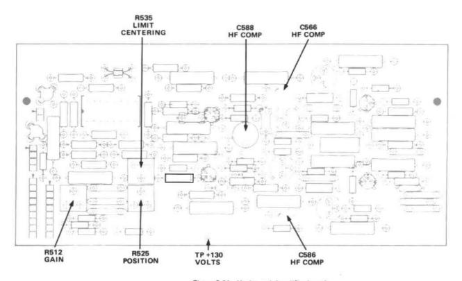
Figure 8-21. Horizontal Amplifier board.
