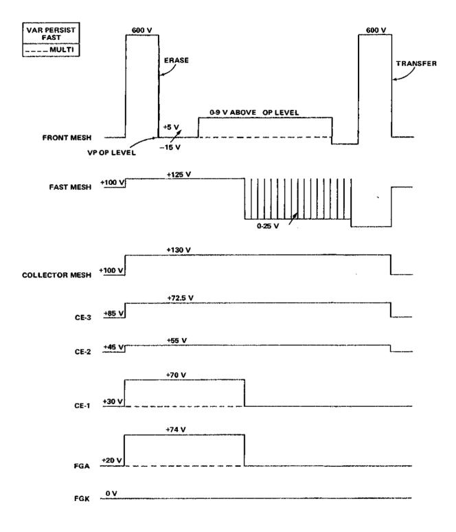
Figure 3-43. FAST VAR PERSIST mode Storage waveforms.
