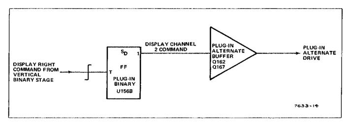
Figure 3-12. Logic diagram of Plug-In Binary and Plug-In Alternate Buffer stage.
