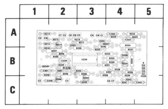
Figure 8-4. A3-Trigger Selector board.
