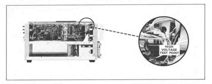
Figure 5-3. Location of High-Voltage Test Point.
