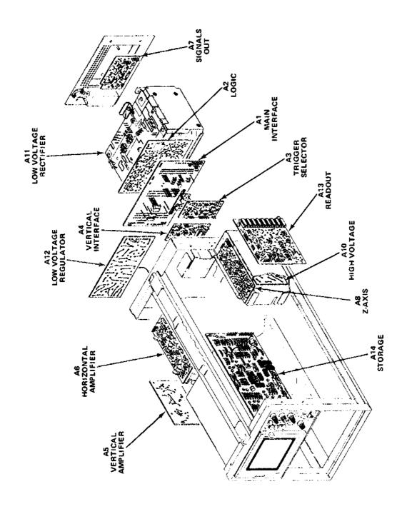
Figure 4-2. Location of circuit boards in the 7623A.
