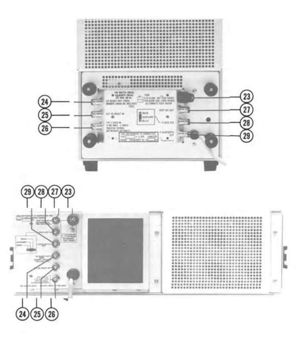
Figure 1-3. Rear panel controls and connectors.
