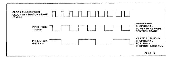
Figure 3-8. Idealized input and output waveforms for Chop Counter stage,
