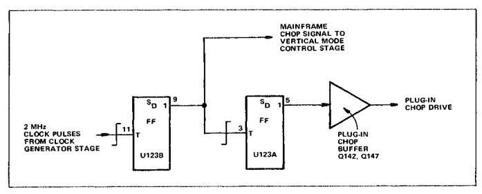
Figure 3-7. Detailed logic diagram of Chop Counter stage.
