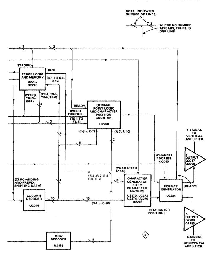
Figure 3-27. Detailed block diagram of the Readout System.
