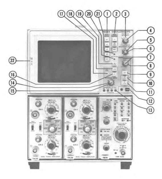
Figure 1-2. Front panel controls and connectors.
