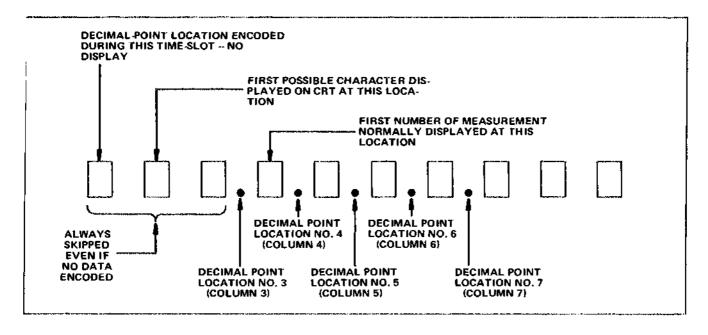
Figure 3-36. Readout word relating 10 possible character locations to the decimal point instructions that can be encoded, and the resultant crt display.
