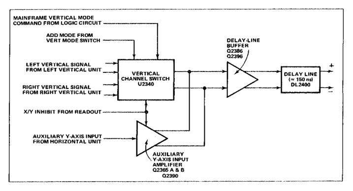
Figure 3-16. Vertical Interface detailed block diagram.
