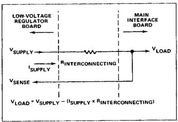
Figure 3-22. Schematic illustrating voltage drop between power supply output and load due to resistance of interconnecting wire.
