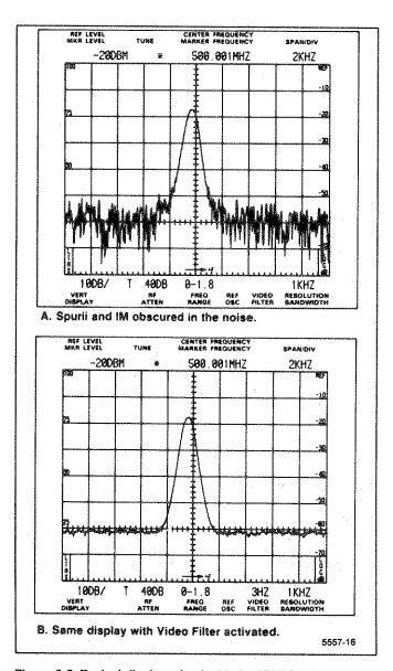
Figure 6-5. Typical display mixed with the VIDEO FILTER.
