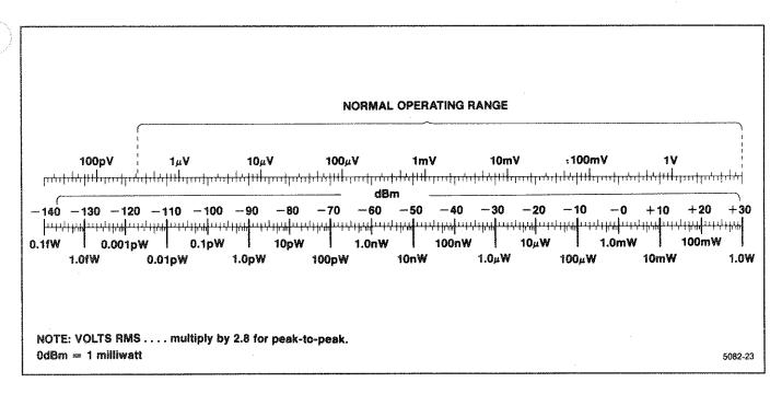
Figure 6-3. Volts-dBm-Watts conversion chart for 50  $\Omega$  impedance.
