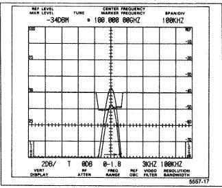
Figure 6-6. Typical display using B-SAVE A to observe the difference between SAVE A and B displays.
