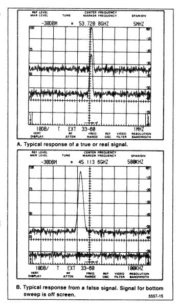
Figure 6-4. Typical example of Identifier mode displays.
