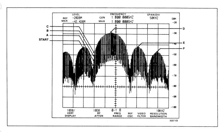
Figure 4-6. Signal finding example.
