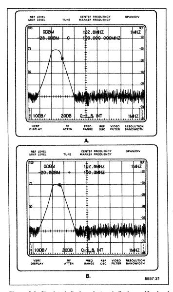
Figure 6-8. Simulated display of stored displays with signal counts. (A) Display when the marker has just been assigned/reassigned to the trace. (B) Display after the marker is tuned.
