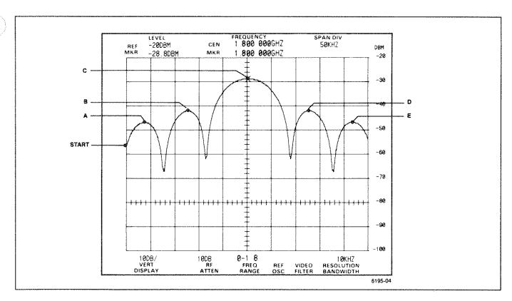
Figure 4-9. Signal finding example.
