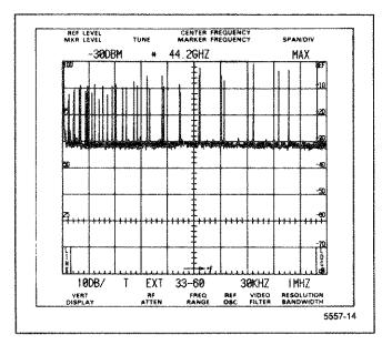
Figure 6-12. A typical display from an external mixer.
