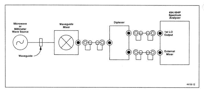
Figure 6-11. Block diagram showing external waveguide mixer installation.
