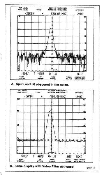
Figure 5-3. Integrating a display with the VIDEO FILTER.
