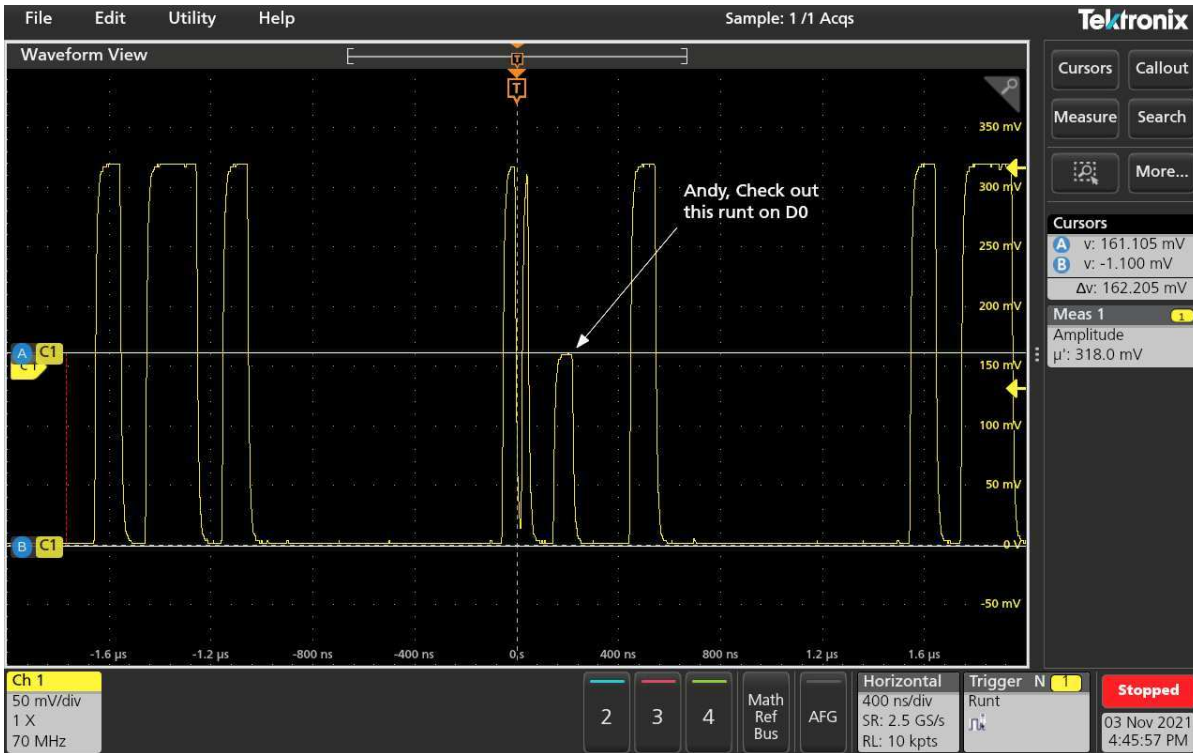
Example of Pulse width trigger used to trigger on a narrow pulse
