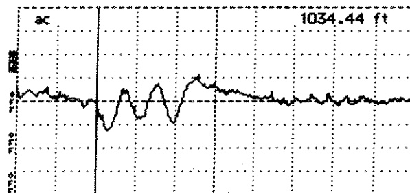
2I - Group of taps expanded (128 avg, 10 ft/DIV, 54.75 dB gain)
