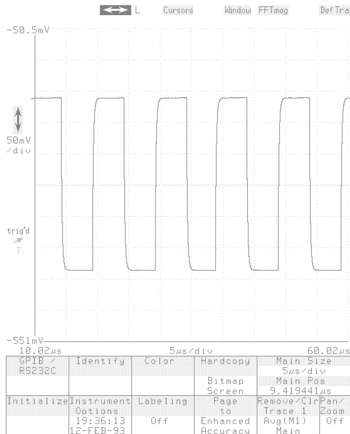
Figure 2-8: The Calibrator Signal After Pressing AUTOSET in Period Mode
