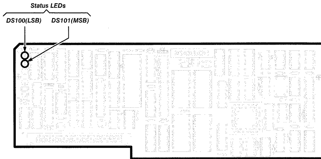
Figure 6-36: A25/A28 Acquisition MPU Board Status LEDs
