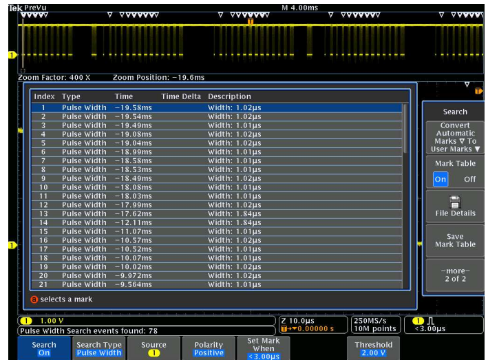
Search step 3: The Search Mark table provides a tabular view of each of the events found by the automated search. Each event is shown with a time stamp making timing measurements between events easy.
