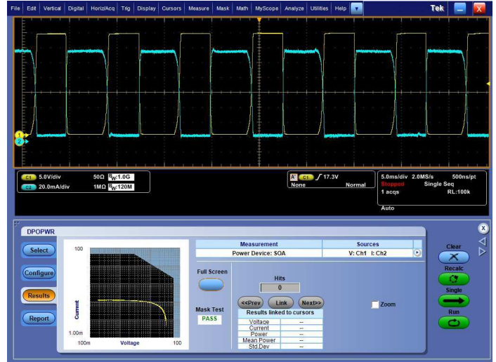
Safe Operating Area measurement. Automated power measurements enable quick and accurate analysis of common power parameters.
