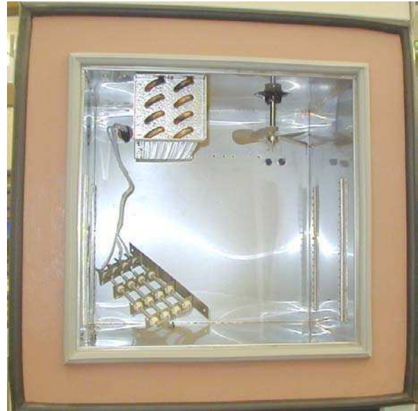
Heater Rack Removal #2
