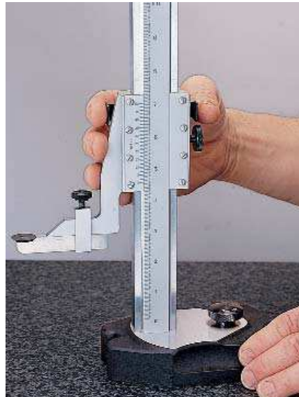
Quick-adjusting screw release permits rapid adjustment of slide to approximate setting followed by precise positioning with fine adjustment knob.
