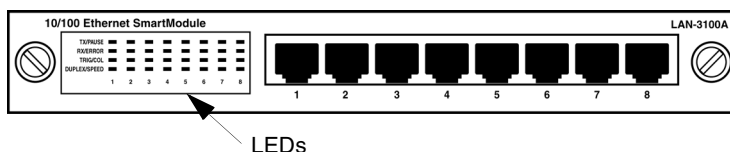
Figure 3-3. Example of LED Locations on an Ethernet Module
