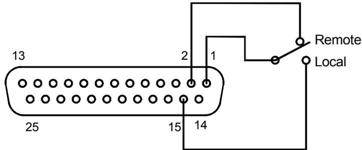
**Figure 2–7 Using Local/Remote Operation with Contact Closure**
