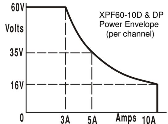
Operating Ranges: Four selectable ranges: 60V/10A, 60V/3A, 16V/10A and Custom Limits.
