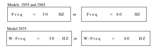
Press the Up or Down Arrow keys to toggle the frequency selection; 50 or 60 hertz, then press the EXIT key to exit to the test mode or toggle to another setting using the SET key.
