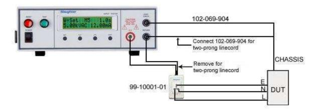
The adapter box allows you an easy way to connect an item which is terminated in a two or three prong line cord. If you are testing a product which is terminated in a three-prong plug, you are also required to perform a continuity or ground bond test on the ground conductor of the DUT to the chassis or dead metal of the product. With the 2900 models, you can perform both the hipot and continuity tests at the same time by activating the continuity function on the instrument.
