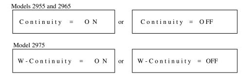
Press the Up/Down Arrow key to select the "ON" or "OFF" function of the Ground Continuity Check mode, the display will show the set status immediately.
