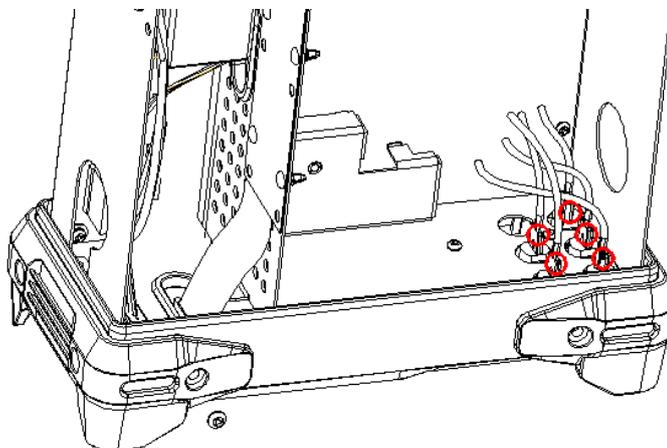
8. Remove the cable and unscrew all the screws then you can remove the PCBA.
