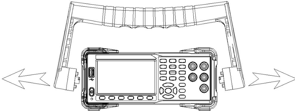
3. Unscrew the four captive screws in the rear bezel and remove the foot pads as indicated by the arrow shown below
