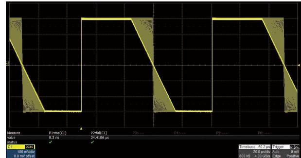
The rise/fall times can be set independently to the minimum of 8.4ns at any frequency and to the maximum of 22.4s. The adjustment step is as small as 100 ps.
