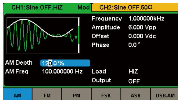
SDG2000X supports plenty of modulation types, such as AM, FM, PM, FSK, ASK, PSK, DSB-AM, and so on. The modulation source can be configured as "Internal" or "External".
