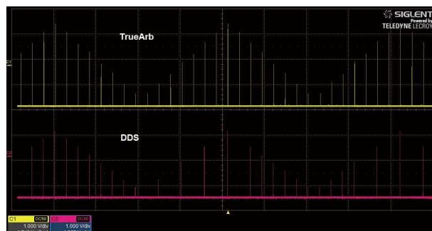
TrueArb generates arbitrary waveforms point by point, never skips any point so that it can reconstruct all the details of the waveform as defined.
