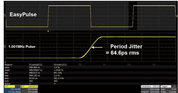
SDG2000X EasyPulse technology effectively overcomes the defect that DDS may cause the one-clock-jitter in arbitrary waveforms.
