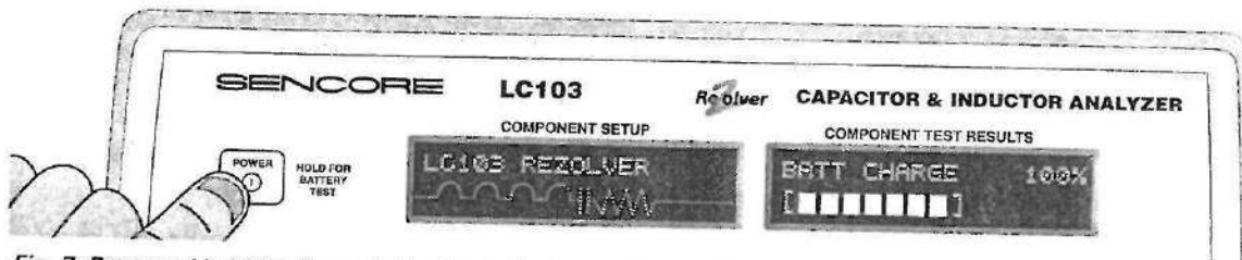
Fig. 7: Press and hold the Power button to read the remaining battery charge.
