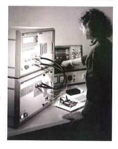
An additional wide range of high current, high voltage pulse generator plug-in networks and external single-and three-phase extension units is available for more demanding industrial test applications. These can be used to create a complete user-defined system for testing to, and beyond, the full IEC, ANSI, IEEE, VDE standards and European Norms.
