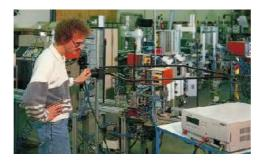
If the instruments and systems to be tested contain magnetically sensitive components then their susceptibility to disruption caused by mains frequency or pulsed-magnetic fields must be checked.
