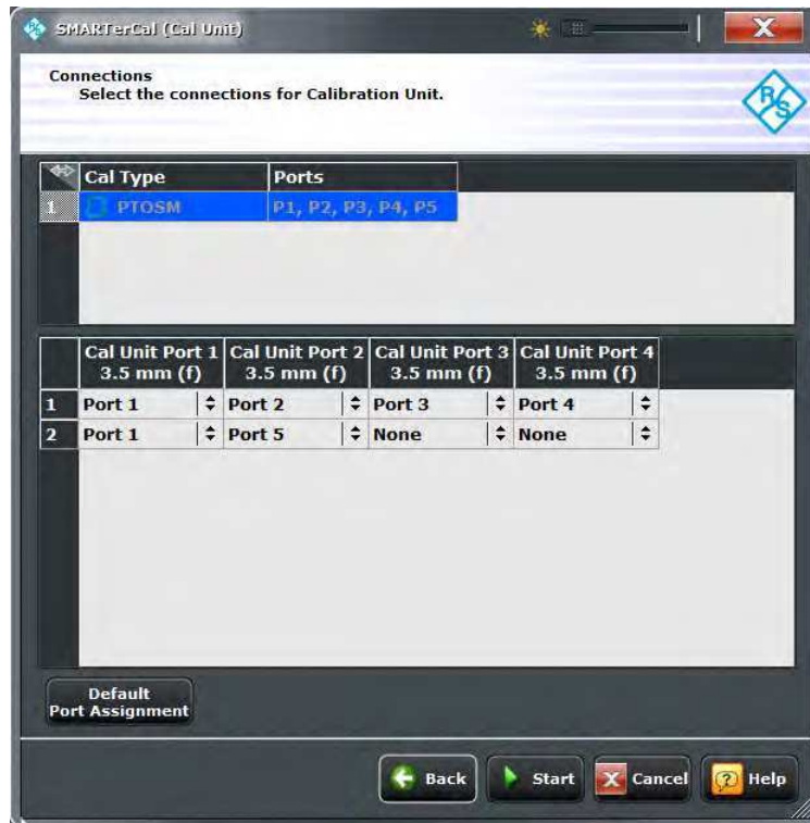
Fig. 4-11: Multiple port assignments
