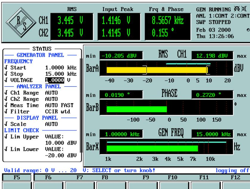
In many cases only a few parameters need to be modified after a measurement sequence has been started. Therefore, entry lines can be selected from the input panels for the generator, analyzer, etc. by means of a checkmark. They are then transferred to a status panel. The status panel thus gives a summary of parameters for a measurement routine, which offers the following advantages:
