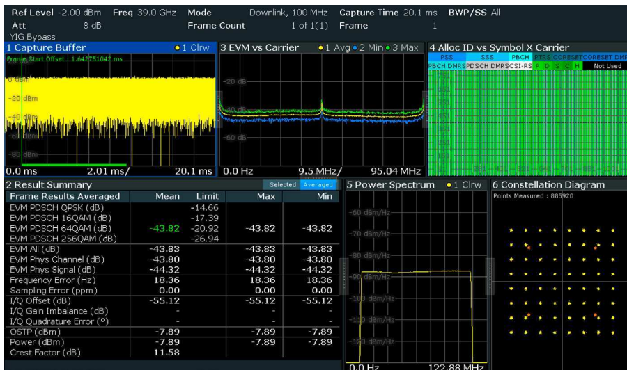
Measured EVM of a 5G NR signal (100 MHz channel bandwidth, 64QAM PDSCH, 39 GHz carrier frequency).
