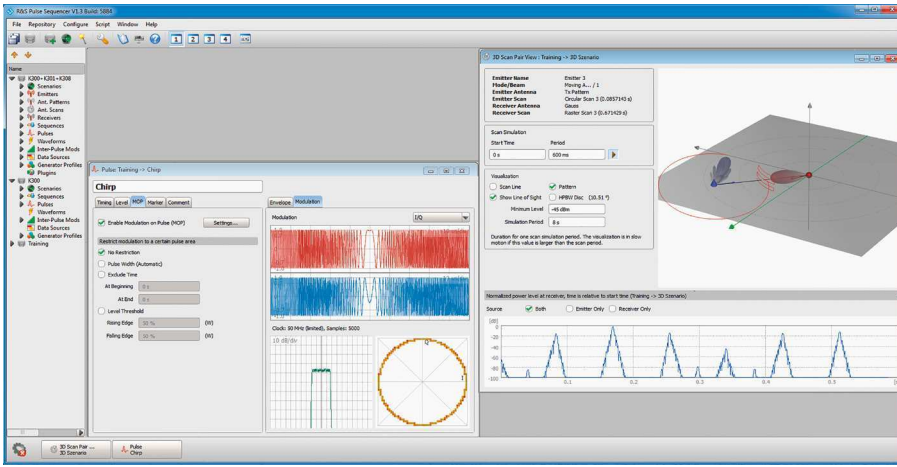
R&S®Pulse Sequencer software for creating radar signals and scenarios with the R&S®SMW200A.
