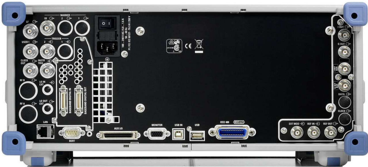
Fig. 2-2: Rear panel view
