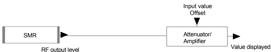
Fig. 4-4 Typical setup with level offset
