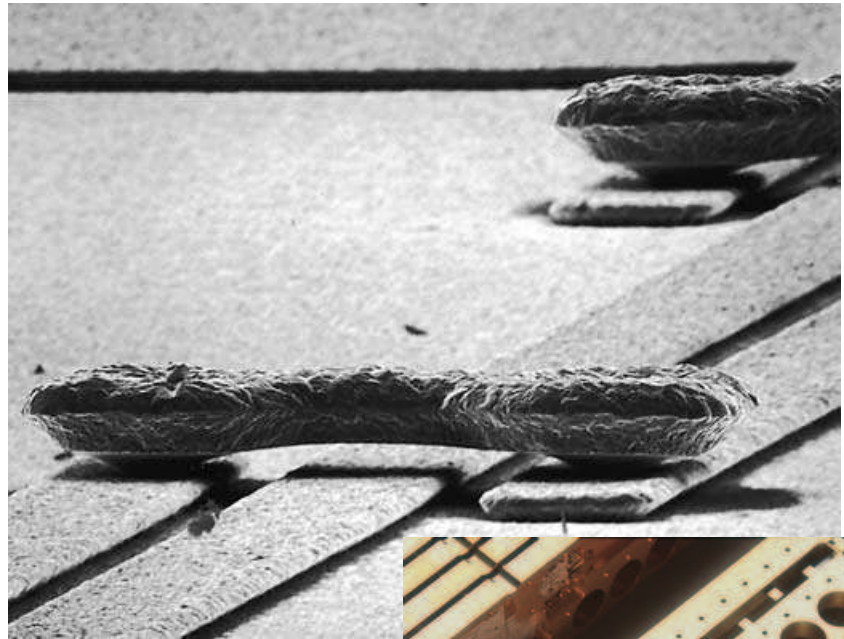
Airbridges is an ideal technique for implementing PCB crossovers with excellent high-frequency characteristics. The photo above has been taken with a scanning electron microscope and shows such an airbridge which is only 0.05 mm long.
