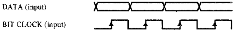
Fig. 2-47 External serial data and bit clock. Data change should take place only on the negative clock edge.
