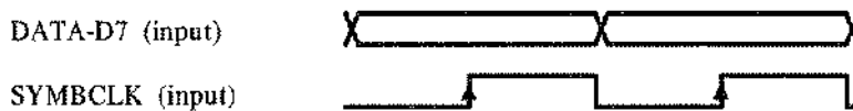
Fig. 2-50 External parallel data and symbol clock. Data change should take place only on the negative clock edge.
