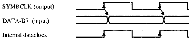
Fig. 2-51 External parallel data and symbol clock. SYMBOL CLOCK = High marks the LSB. A status change of DATA and SYMBOL CLOCK should be performed synchronously.
