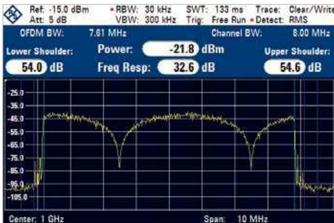
DVB T spectrum exhibiting two deep dips caused by fading.
