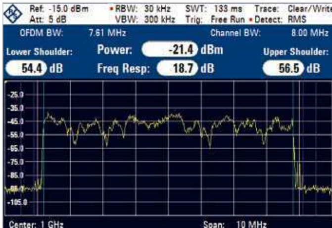
Typical DVB T spectrum distortion obtained with the TU6 channel model.
