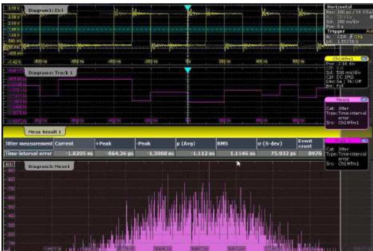
Figure 16-1: TIE measurement with CDR trigger, 10 Mbps, with track and histogram
