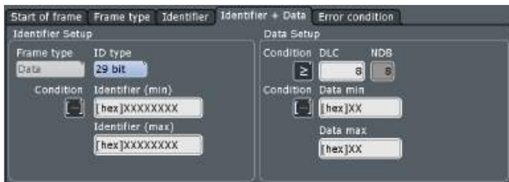
Figure 12-26: Identifier + Data search setup for CAN signals
