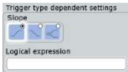
Figure 13-1: Edge trigger settings for trigger source = logical combination of digital channels (Logic)
