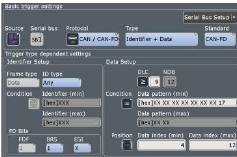
Figure 12-21: Trigger setup to trigger on data byte with value = 17 at 11th data byte location
