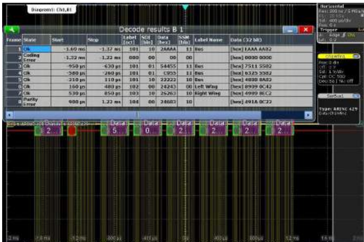
Figure 12-51: Decoded ARINC 429 signal with applied label list and results table. The second and eighth frame contain errors.
