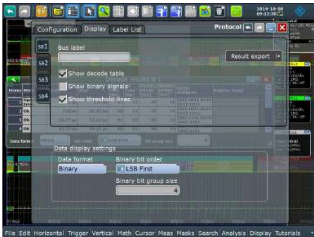
Figure 12-104: The data display settings can be configured in the Display tab of the Protocol dialog
