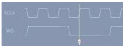
Figure 12-39: Word select trigger on I 2 S standard signal with clock polarity "Rising" and "Normal" WS polarity (left = 0)
