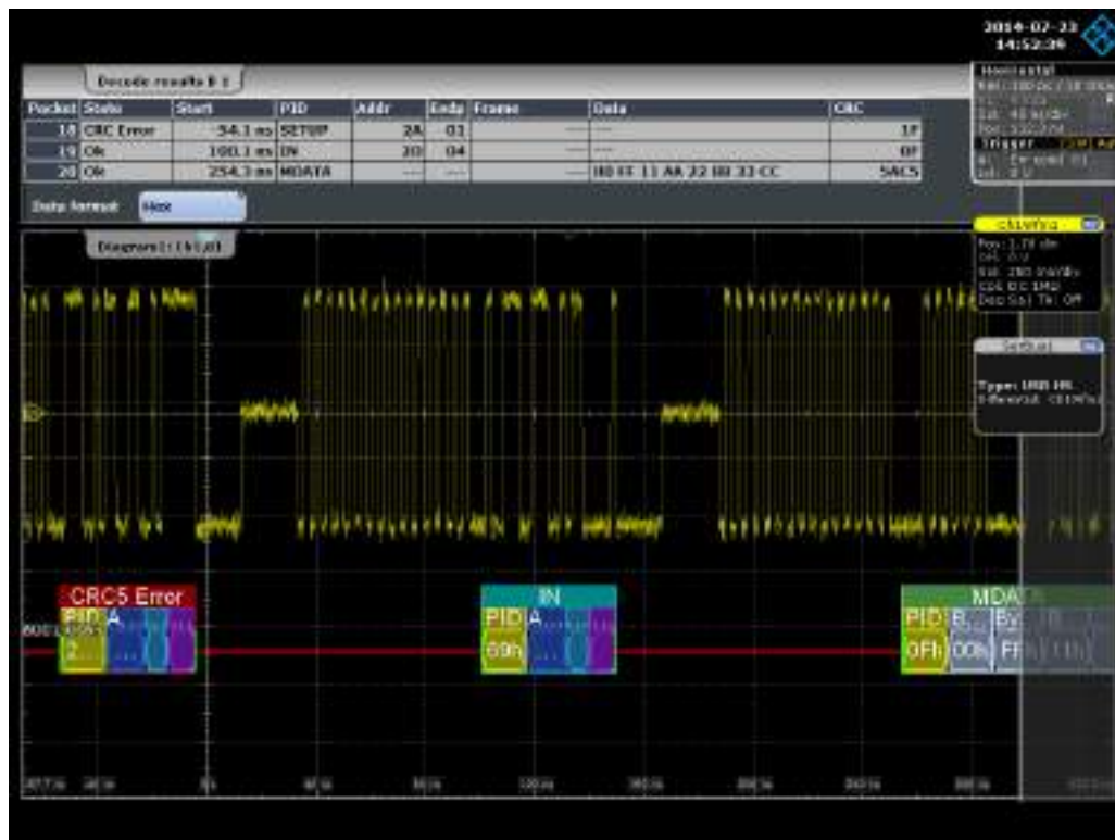
Figure 12-116: USB high speed protocol: decoded and binary signal, and decode results
