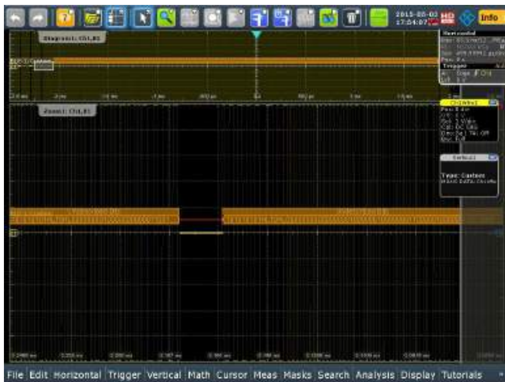
Figure 12-98: The function "Undescribed Bits" catches frames missed by the frame format descriptions
