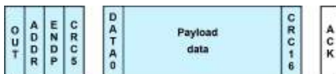
Figure 12-107: Example of a bulk OUT transfer. Blue: host speaks, white: device speaks
