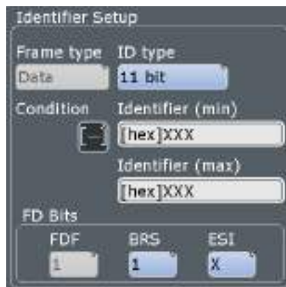
Figure 12-14: Identifier setup for CAN FD
