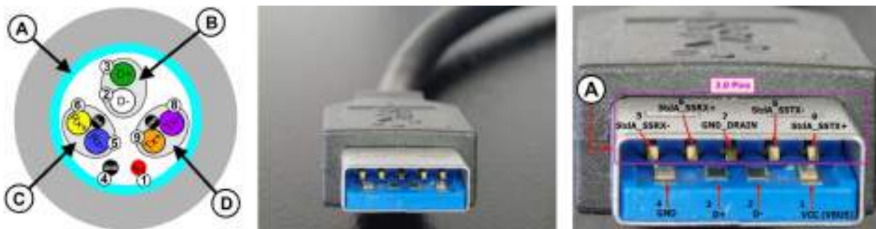
Figure 12-118: USB 3.1 cable cross-section and Standard-A plug - backward compatible with USB 2.0
