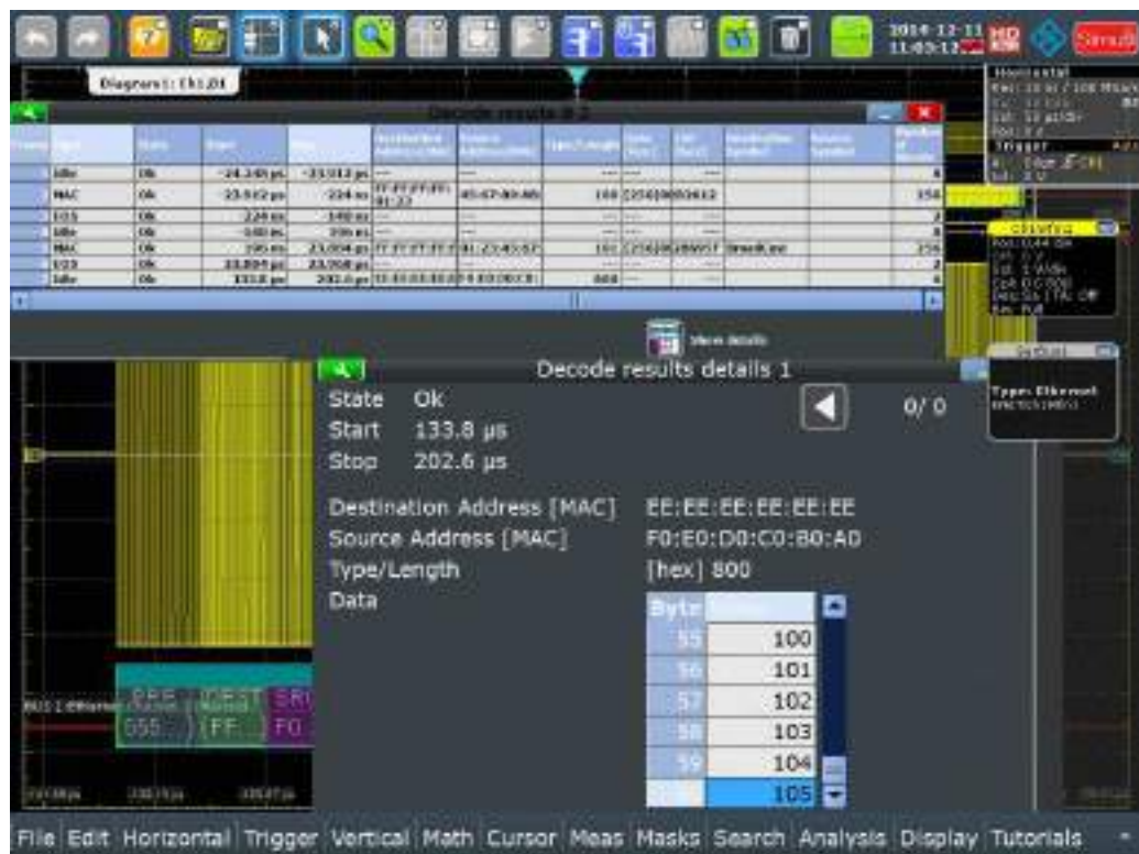
Figure 12-56: Ethernet 10BASE-T: decoded and binary signal, with decode results table and details
