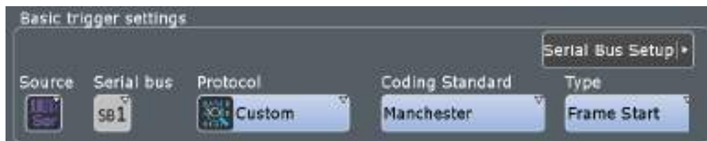
Figure 12-94: Custom serial bus trigger event settings dialog (here with "Manchester" and "Frame Start" selected)
