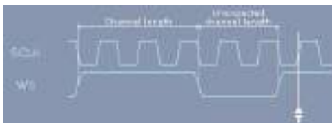
Figure 12-38: Trigger on errors in I 2 S standard signal with clock polarity "Rising"
