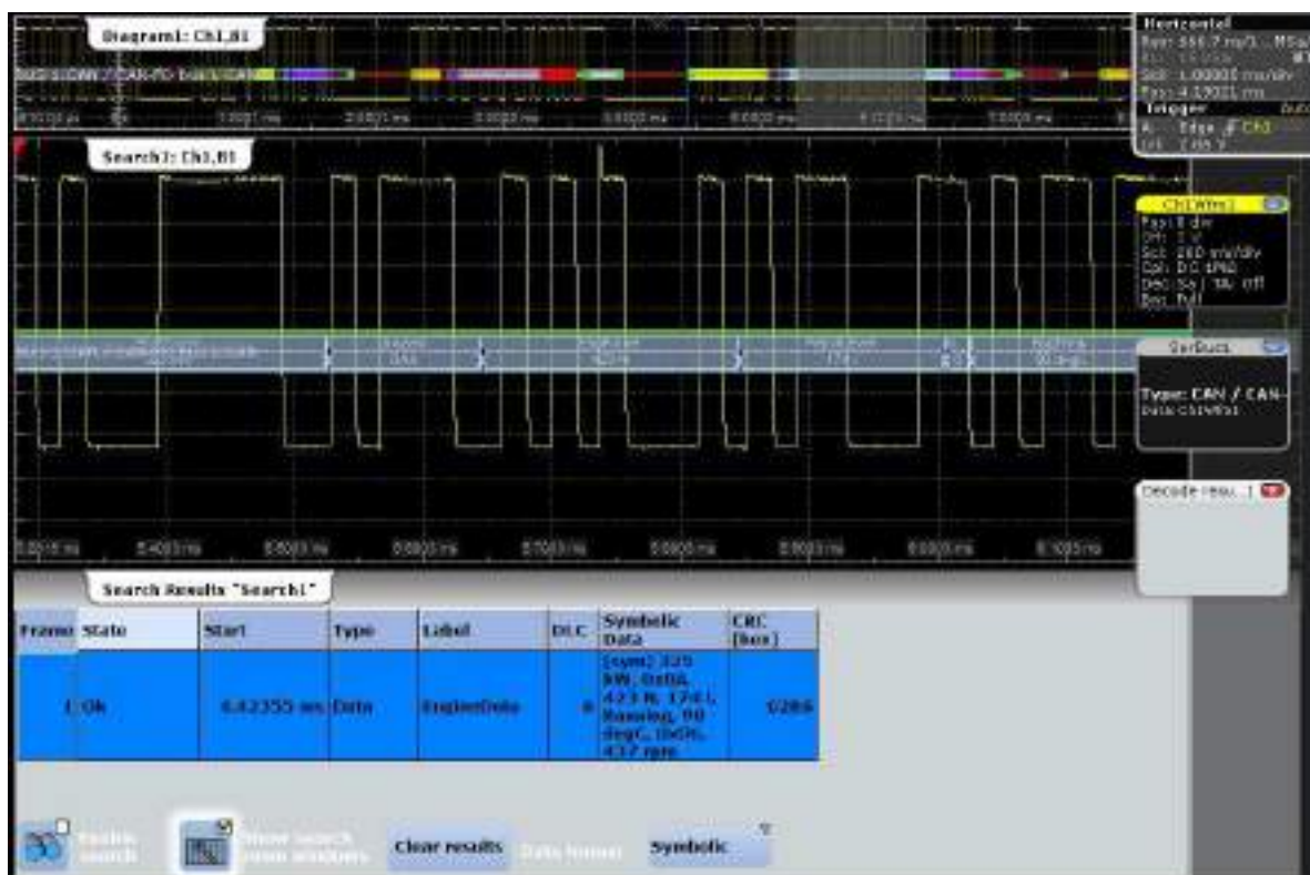
Figure 12-31: Search results table and search zoom window. Search for signal "IdleRunning" with value "Running" (bit value = 0)
