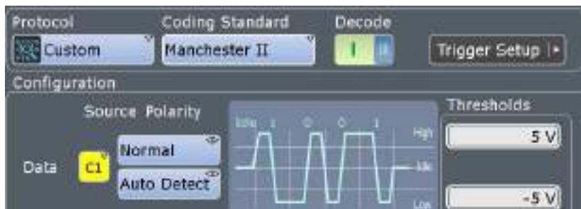
Figure 12-85: Custom serial bus coding configuration Manchester II
