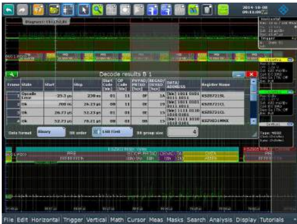
Figure 12-103: The same signal trace and decode results table as in the previous figure, but only with "DATA" in binary format
