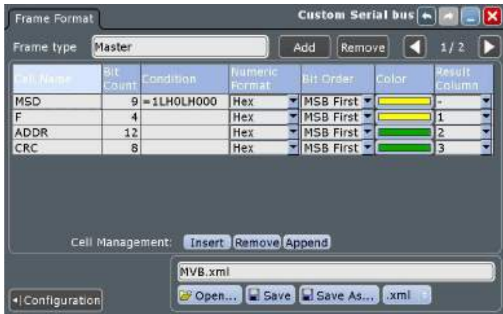
Figure 12-89: Example of a custom "MVB" frame format description (frame 1 of 2)
