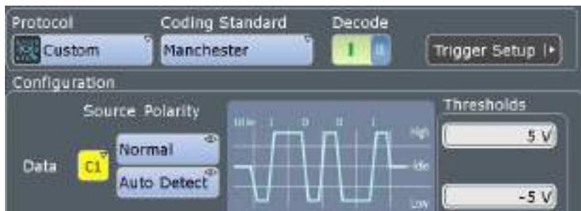
Figure 12-84: Custom serial bus coding configuration Manchester
