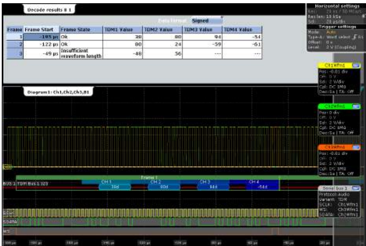
Figure 12-41: Decoded TDM signal with 4 channels, frame offset 16 bit, channel offset 4 bit, word length 8 bit and inverted FSYNC and SDATA polarity
