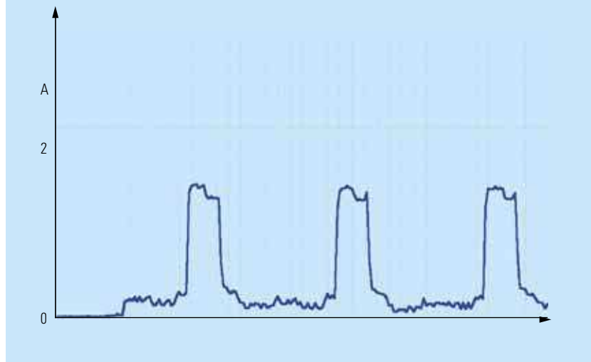
Dynamic current drain of critical GSM mobile phone, measured with NGMO2
