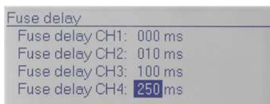
Figure 4-5: Fuse delay (example R&S HMP4040)
