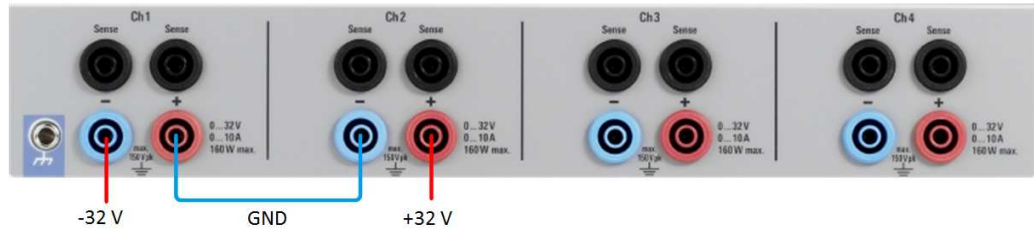
Figure 5-5: Example of a multi-quadrant connection
