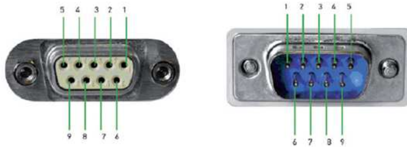
Figure B-2: RS232 Pin Assignment
