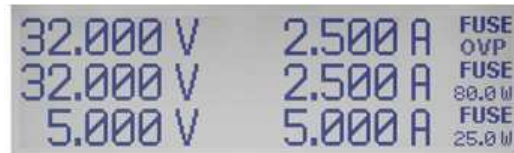
Figure 4-6: Overvoltage protection (example R&S HMP2030)
