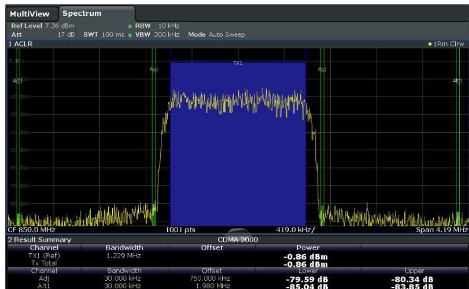
Figure 6-30: Adjacent channel power measurement on a CDMA2000 1x signal
