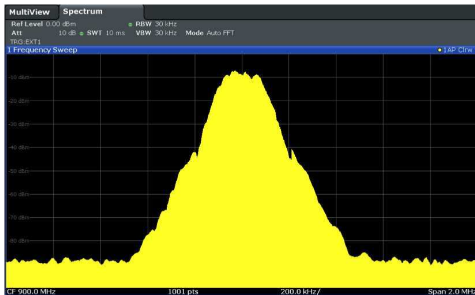
Figure 7-29: GSM signal with GATE OFF
