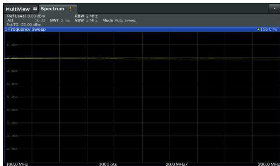
Figure 7-7: Measurement results from generator, analyzer and connecting cables
