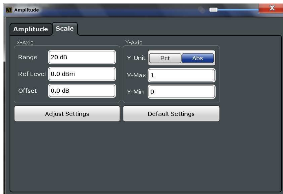
Figure 6-41: Scale settings for CCDF diagram
