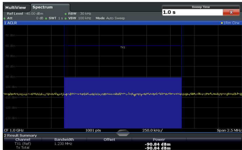
Figure 6-33: Measurement of the R&S FSW's intrinsic noise power in a 1.23 MHz channel bandwidth.
