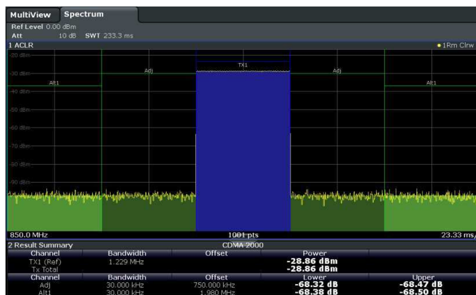
Figure 6-21: Measuring the channel power and adjacent channel power ratio for CDMA2000 signals with zero span (Fast ACLR)
