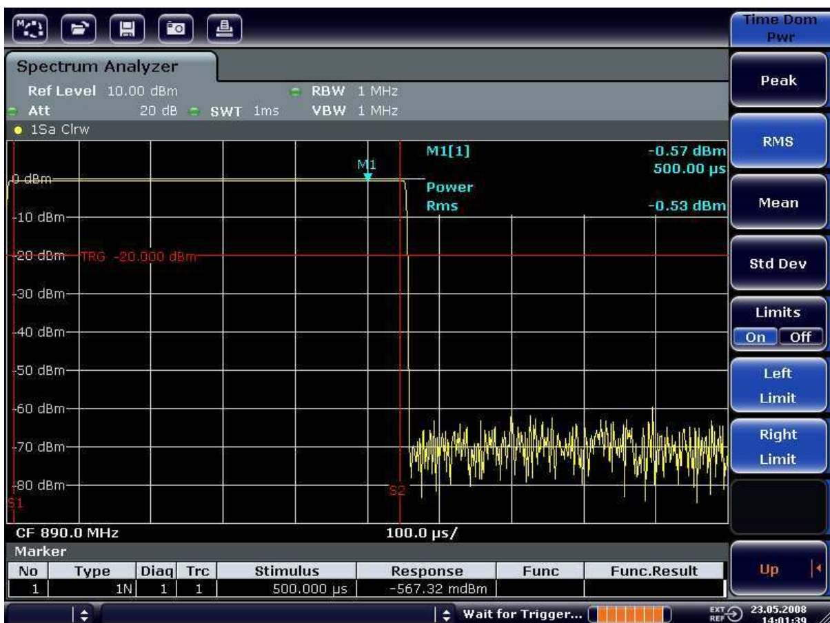
Fig. 2-18: Measurement of the average power during the burst of a GSM signal
