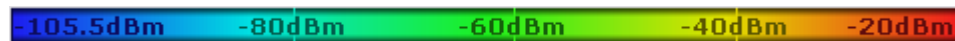
Fig. 3-49: Linear color curve shape = 0; colors are distributed evenly over the complete result range
