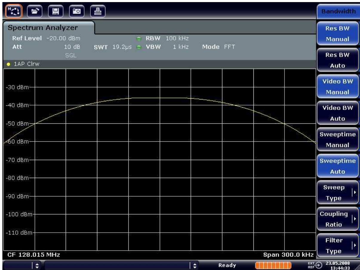
Fig. 2-15: Measurement of two equally-leveled RF sinusoidal signals with a resolution bandwidth which is larger than their frequency spacing
