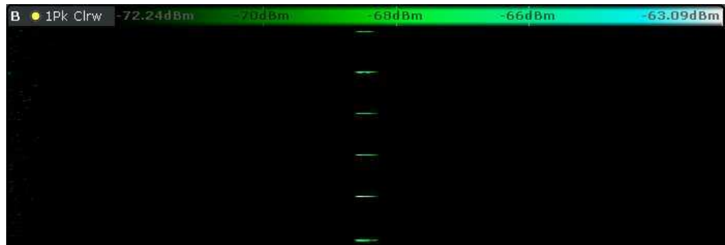
Fig. 3-6: Spectrogram that shows the peaks of a pulsed signal only
