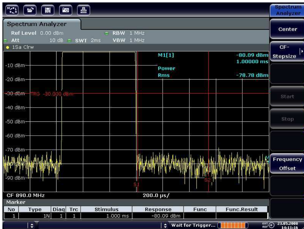
Fig. 6-21: Display of the filter edge of the 300 kHz filter as an FM discriminator characteristic
