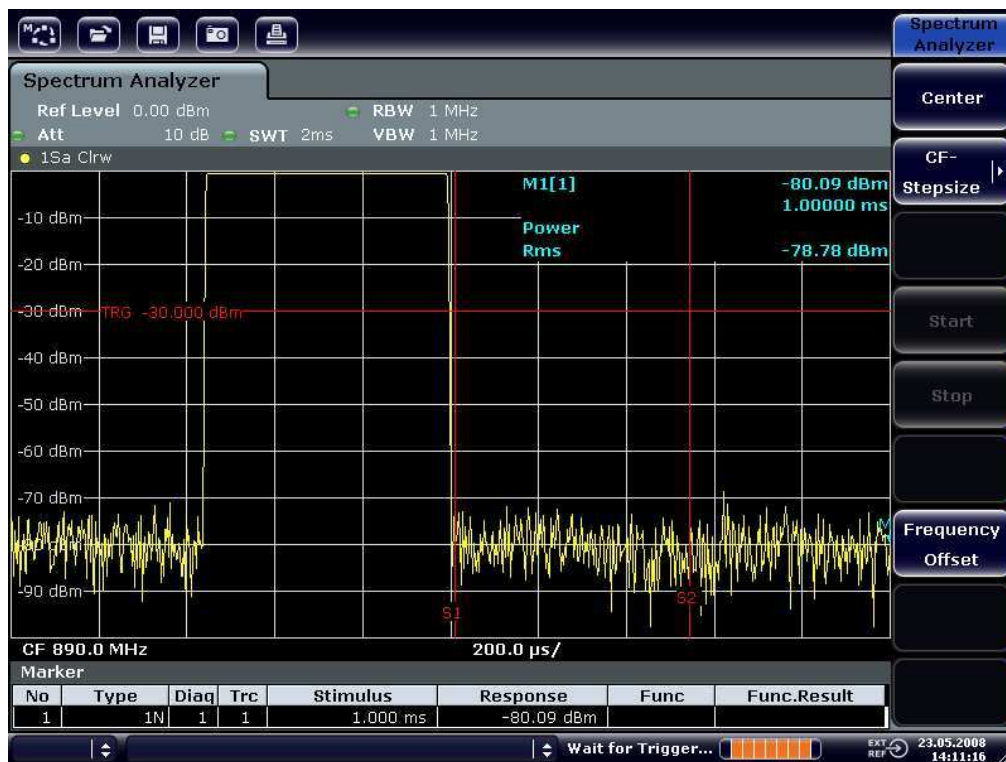
Fig. 6-20: Measurement of the signal-to-noise ratio of a GSM burst signal in zero span.
