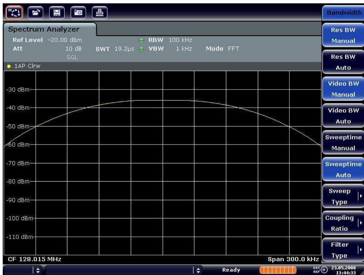
Fig. 6-13: Measurement of two equally-leveled RF sinusoidal signals with a resolution bandwidth which is larger than their frequency spacing
