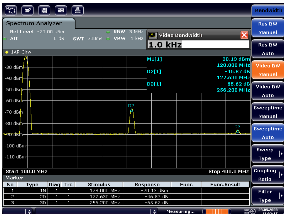
Fig. 6-11: Suppression of noise during harmonics measurement by reducing video bandwidth
