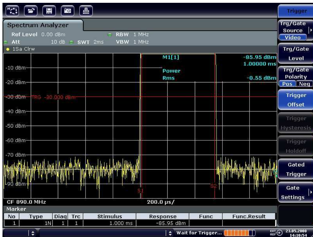
Fig. 6-19: Power measurement during the activation phase of the burst
