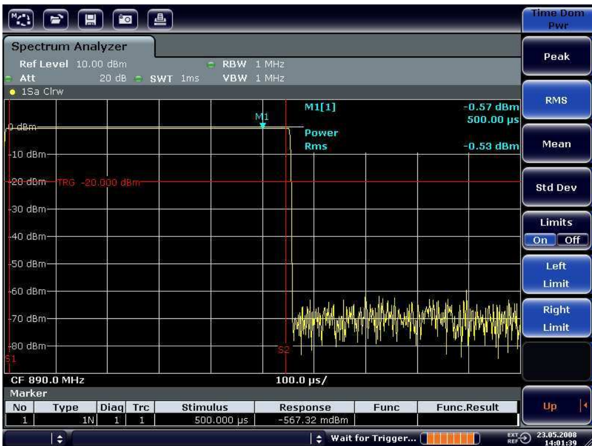
Fig. 6-16: Measurement of the average power during the burst of a GSM signal
