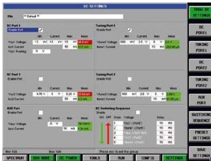
Menu for setting the DC ports for signal source analysis and additional port for negative supply voltage.
