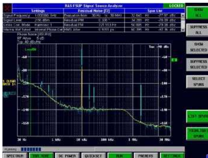
Interference can be identified (vertical blue lines) and listed.
