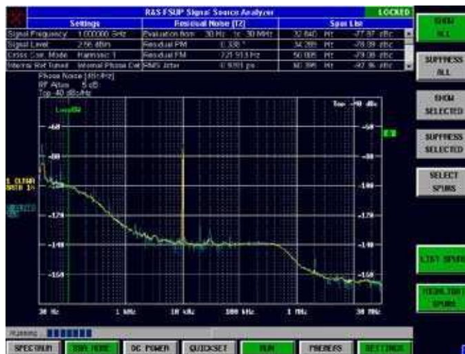
Typical phase noise measurement with phase detector method – signal frequency, level, and residual noise are displayed.
