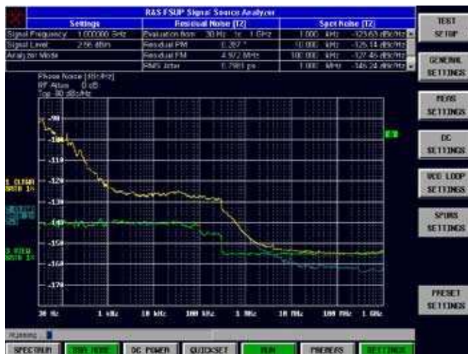
Measurement of phase noise using the spectrum analyzer method. The blue trace shows the measurement result up to an offset frequency of 1 GHz, the inherent noise of the system (green trace) is subtracted from the original measurement (yellow trace).
