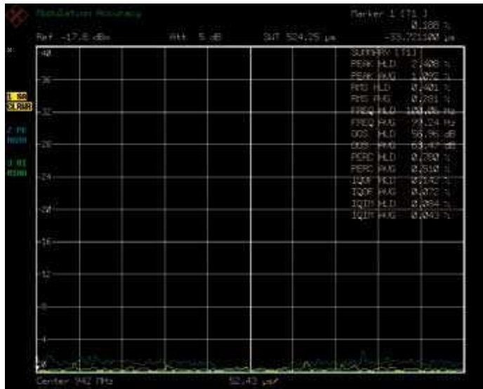
Measurement of modulation accuracy on EDGE burst.
