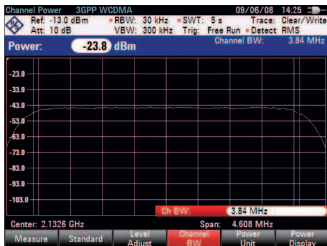
Channel power measurement.
