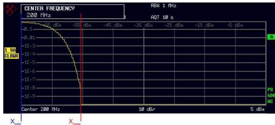
Fig. 4.29 APD of receiver noise
