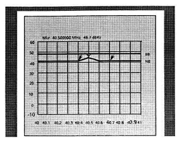
Fig. 3-95 Detuning method: narrowband interference with superimposed broadband interference, measured at a test bandwidth of 100 kHz and a stepsize of 50 kHz. The decisive adjacent levels are marked. For illustration, the extension of the frequency axis is substantially larger than using marker zoom.
