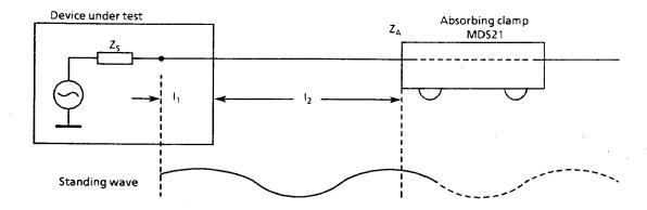
Fig. 3-78 Impedances  $Z_S$  and  $Z_A$  and lengths of the lines  $I_1$  und  $I_2$  with RFI power measurement.  $Z_S$ ,  $Z_A$  and  $I_1$  are nearly constant within one subrange; it is thus sufficient to determine the local maximum  $I_2$  of the subrange maximum.
