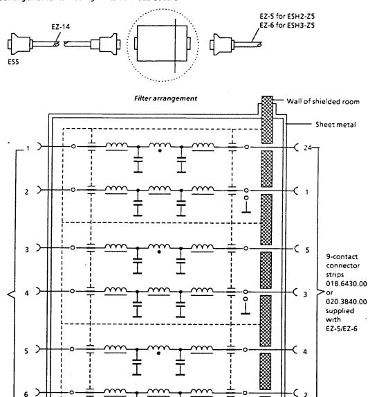
Fig. 3-72 Arrangement of connecting cables EZ-5, 6 and 14 with lowpass filters to provide the 5-V supply and control information for artificial mains networks ESH2-Z5 and ESH2-Z5 in a shielded room.
