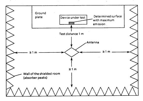
Fig. 3-100 Test setup for the measurement of interference fieldstrengths
