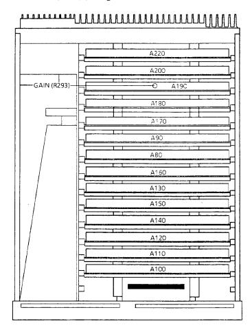
Fig. 4-10 Position of the potentiomenter GAIN R293
