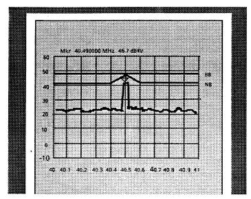
Fig. 3-98 Narrowband interference with superimposed broadband interference, measured at a bandwidth of 100 kHz (upper curve) and measured again at a bandwidth of 10 kHz (lower curve). The highest value of the broadband measurement is compared with the highest value of the narrowband measurement.
