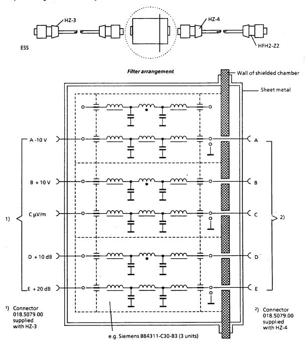
Fig. 3-84 Arrangement of connecting cables HZ-3/4 with AF filters for supplying and coding active antenna HFH2-Z2 in shielded rooms
