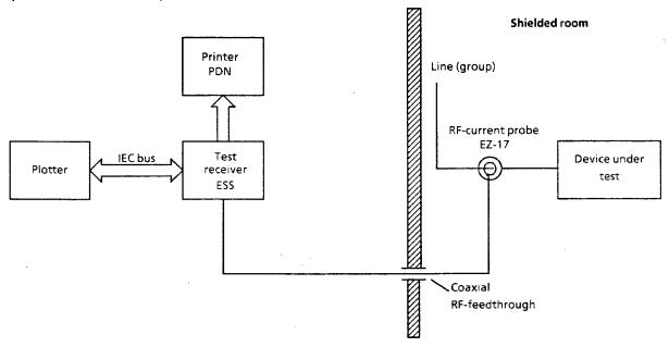
Fig. 3-77 Block diagram of a test setup with RF-current probe EZ-Z17 and device under test in a shielded chamber
