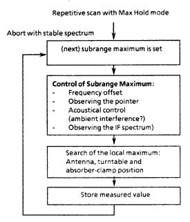
Fig. 3-65 Sequence scheme for the measurement of instable interferences
