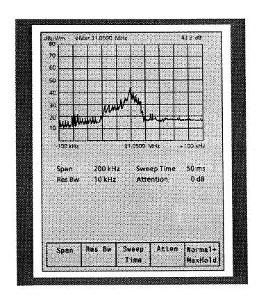
Fig. 3-68 IF analysis spectrum with marker frequency of Fig. 3-67
