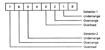
Fig. 3-62 Format of the validity byte with unformatted output of scan results.
