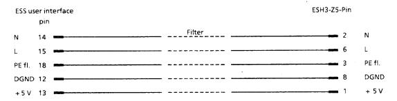
Fig. 3-67 Connection between ESS and ESH3-Z5 (cable EZ-14)
