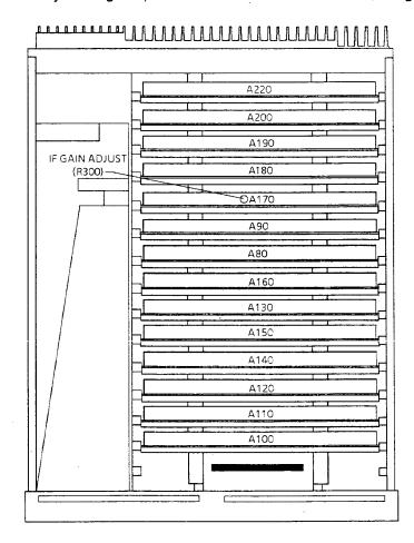
Fig. 4-8 Position of the potentiometer IF GAIN ADJUST, R300 (instrument seen from above)
