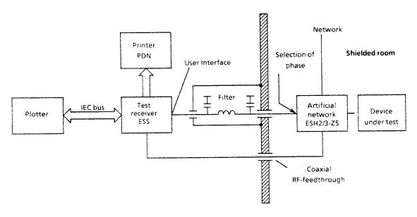
Fig. 3-65 Block diagram of a test setup with artificial mains network and device under test in a shielded room
