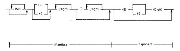
Fig. 3-50 Syntax diagram of messages sent by the receiver
