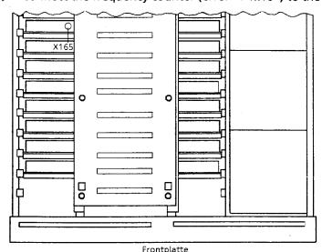
Fig. 4-1 Location of the socket X165 (instrument seen from below)
