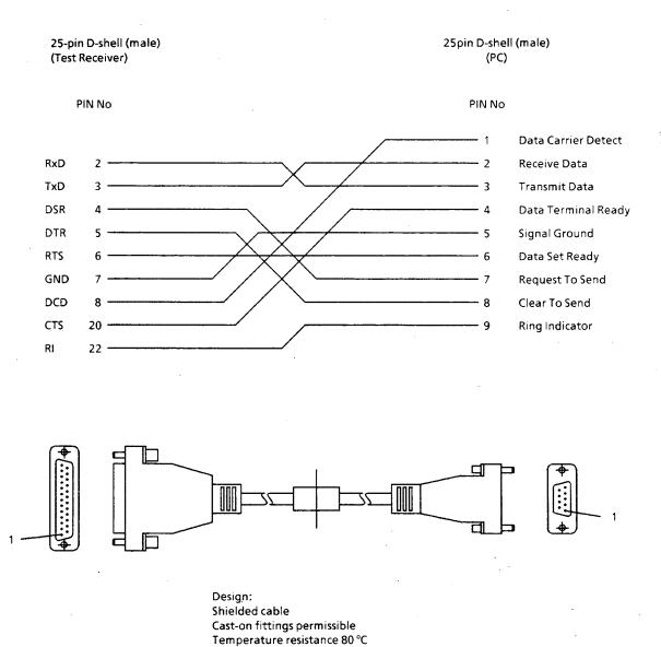
Fig. 4-12 Adapter cable for serial interface
