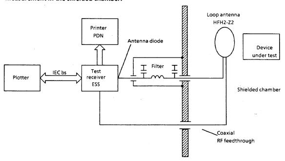
Fig. 3-83 Block diagram of a test setup including loop antenna HFH2-Z2 and device under test in the shielded chamber
