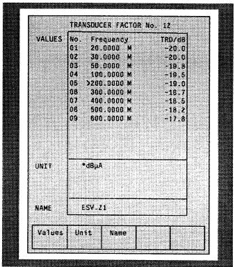
Fig. 3-12 List for transducer factor
