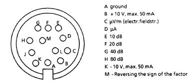
Fig. 3-44 Assignment of the 12-contact Tuchel-type female connector
