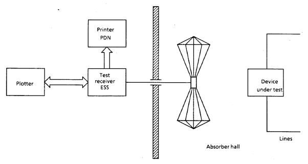
Fig. 3-86 Test setup for RFI fieldstrength measurement in an absorber hall.
