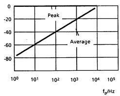
Fig. 3-96 Peak and linear average value indication as a function of the pulse frequency of an interference at a test bandwidth of 10 kHz
