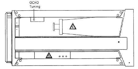
Fig. 4-3 Position of potentiometer OCXO TUNING, R368 (lateral view on instrument)
