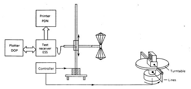
Fig. 3-87 Test setup for free-field RFI fieldstrength measurement
