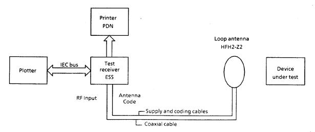
Fig. 3-85 Block diagram of a test setup with open air test. Make sure that the antenna is decoupled from printer and plotter, e.g. by grounding the cable insulation wall and by means of sheeth current stop filters.
