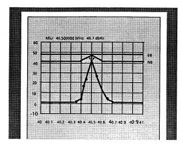
Fig. 3-97 Peak and linear average value indication of a narrowband interference with superimposed broadband interference
