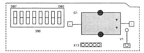
Fig. 4-4 Mounting position of the battery and DIP switch S90 for setting of the receiver configuration (cf. section 4.3.4)
