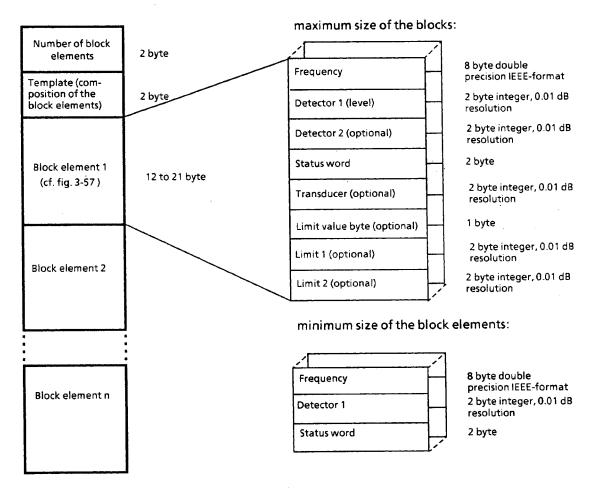
Fig. 3-59 Composition of a data block in binary format
