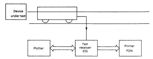
Fig. 3-79 Block diagram of a test setup with MDS clamp and device under test in a shielded room
