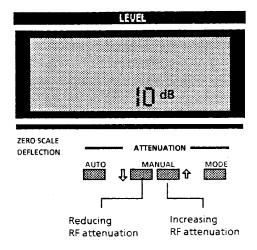
The RF attenuation selected is shown in the LEVEL display.
