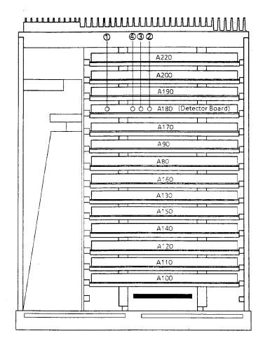
Fig. 4-9 Position of the adjustment points for the DETECTOR BOARD module
