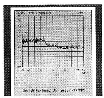
Fig. 3-67 Zoomed RF analysis spectrum with marker frequency of Fig. 3-66
