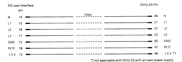
Fig. 3-66 Connection between ESS and ESH2-Z5 (cable EZ-13)
