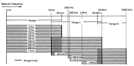
Fig. 3-4 Receiver frequencies in relation to settable IF bandwidths
