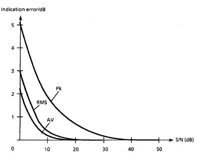
Fig. 3-6 Increase in indication of an unmodulated sinusoidal signal as a result of noise as a function of the signal-to-noise ratio.
