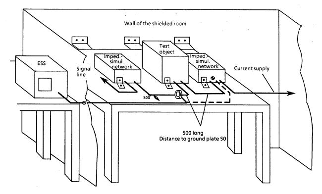
Fig. 3-99 Test setup for the measurement of interference currents and interference voltages
