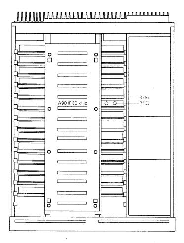
Fig. 4-11 Position of the potentiometers R153 and R387
