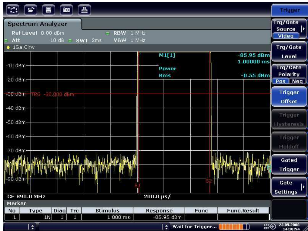
Figure 3-18: Power measurement during the activation phase of the burst
