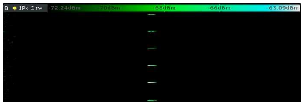
Figure 5-2: Spectrogram that shows the peaks of a pulsed signal only
