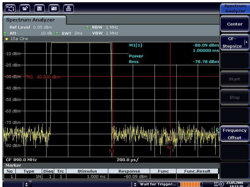
Figure 3-20: Display of the filter edge of the 300 kHz filter as an FM discriminator characteristic
