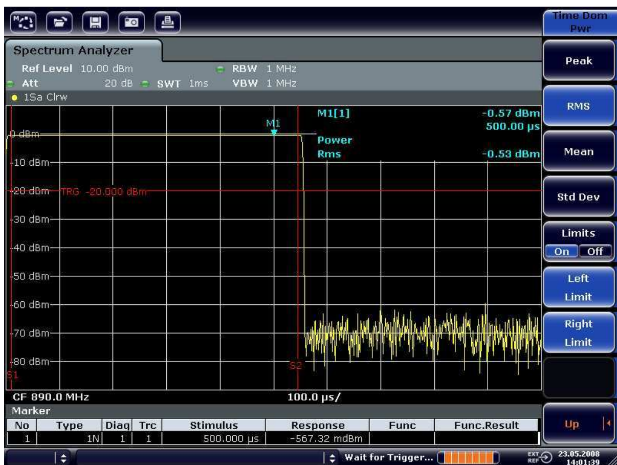
Figure 3-15: Measurement of the average power during the burst of a GSM signal
