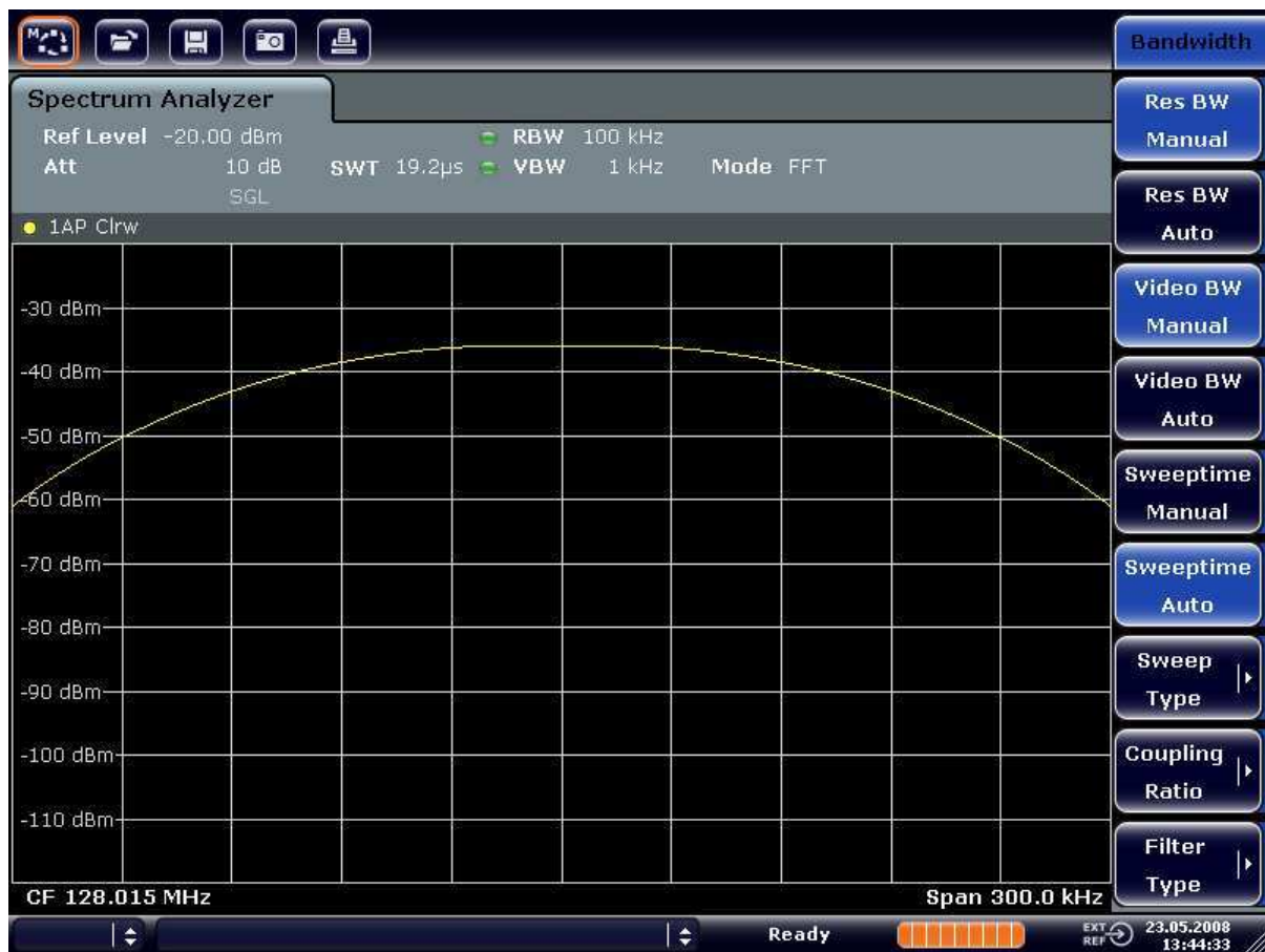
Figure 7-5: Measurement of two equally-leveled RF sinusoidal signals with a resolution bandwidth which is larger than their frequency spacing
