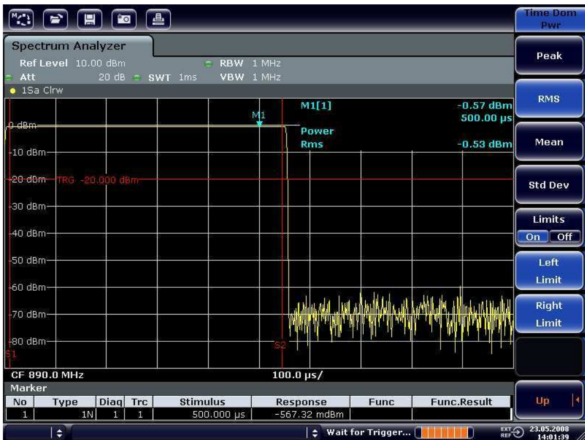
Figure 7-8: Measurement of the average power during the burst of a GSM signal
