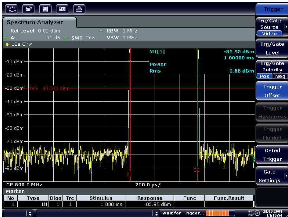
Figure 7-11: Power measurement during the activation phase of the burst
