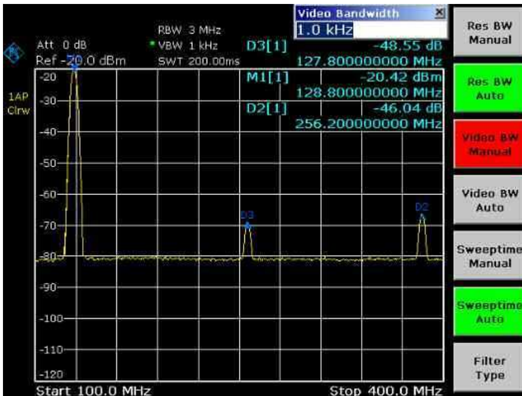
Fig. 5–3 Suppression of noise during harmonics measurement by reducing video bandwidth
