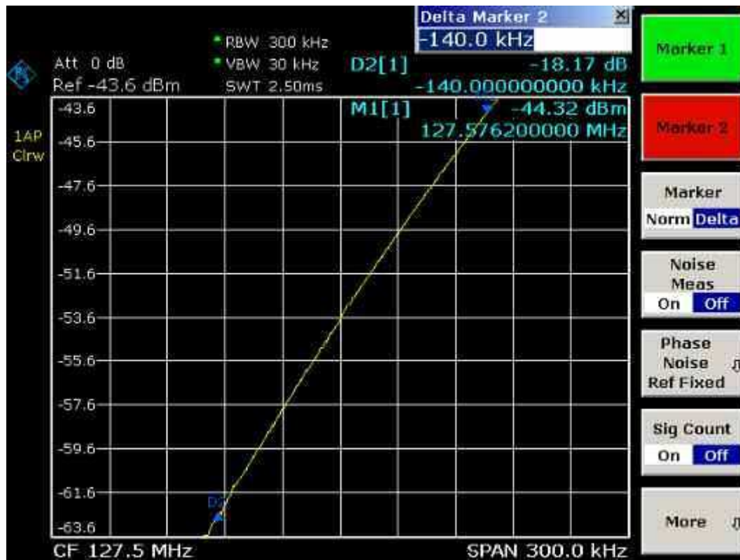
Fig. 5–14 Display of the filter edge of the 300 kHz filter as an FM discriminator characteristic
