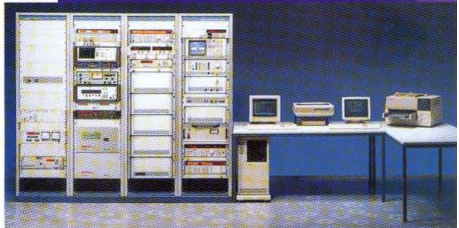
Type approval of GSM mobiles, using very comprehensive RF and audio tests, is performed exclusively by the Rohde & Schwarz System Simulator
