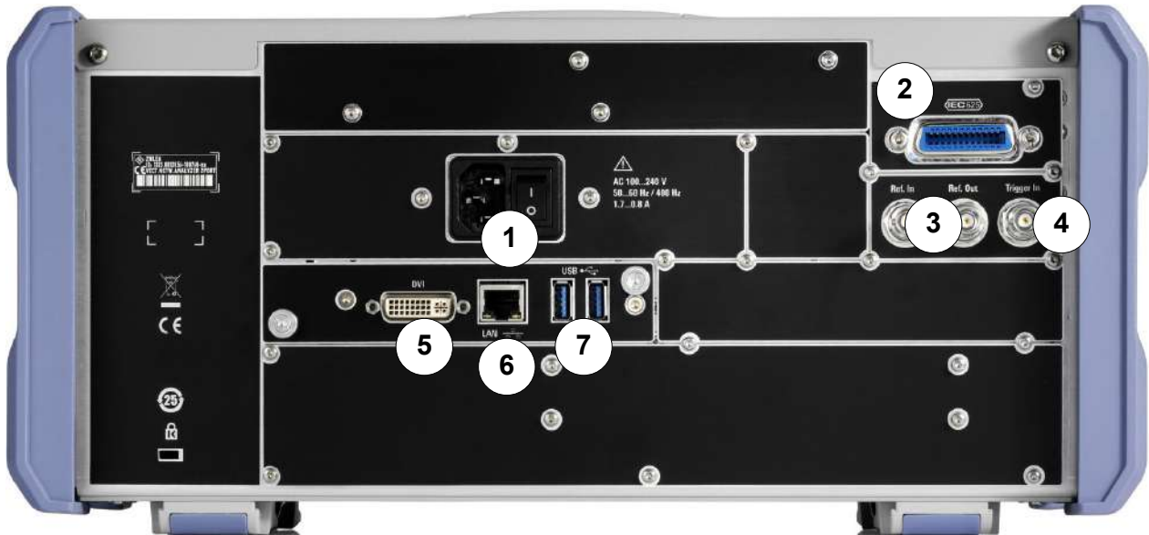
Figure 4-4: Rear panel view R&S ZNLE
