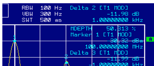
Fig. 5-15 Measurement of the AM modulation depth. The modulation depth shown is MDEPTH. The frequency of the AF signal can be obtained from the frequency display of the delta marker.
