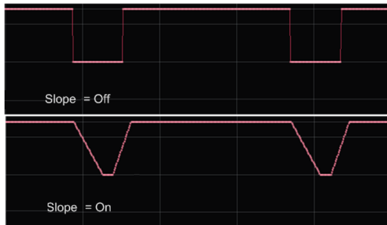
Figure 5-1: Impact of the "Slope" parameter ("RLC Curve" = Off)
