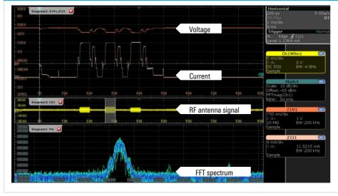
The multi-channel probe helps to correlate multidomain measurements with high dynamic range, e.g. voltage, current, RF signals and power.
