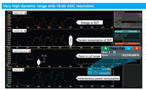
The extraordinarily high dynamic range allows the measurement of both active state currents and sleep currents, in this example 12 mA and 30 µA. Automated measurements make it possible to calculate the total energy consumption.
