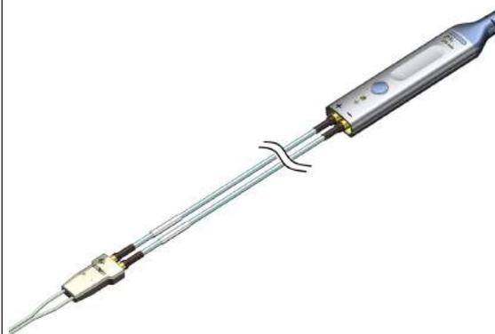
The R&S RT-ZMA11 tip cable solder-in ET cannot be plugged directly into the probe amplifier. Always connect the R&S RT-ZMA11 tip cable solder-in ET to the 1-m extension cable pair and connect the other end of the extension cable pair to the R&S RT-ZM probe amplifier.
