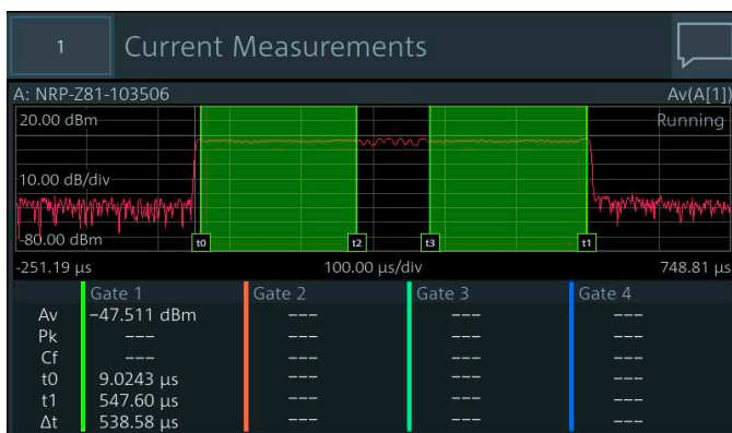
Determination of power of an EDGE burst using an R&S®NRPxxS(N) three-path diode power sensor and the gate function; exclusion of training sequence in the center of the signal
