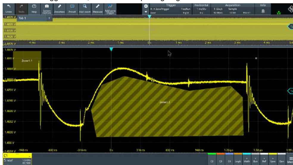
Figure 7-8: Zoom on a zone trigger in the mV and ns range
