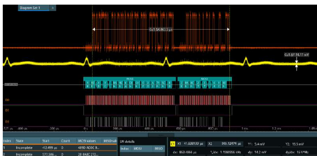
Figure 13-3: Decoded and binary SPI signal
