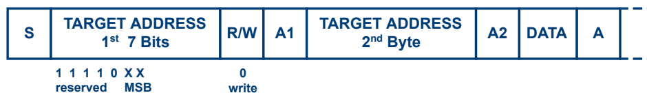
Figure 13-7: 10-bit address, write access
