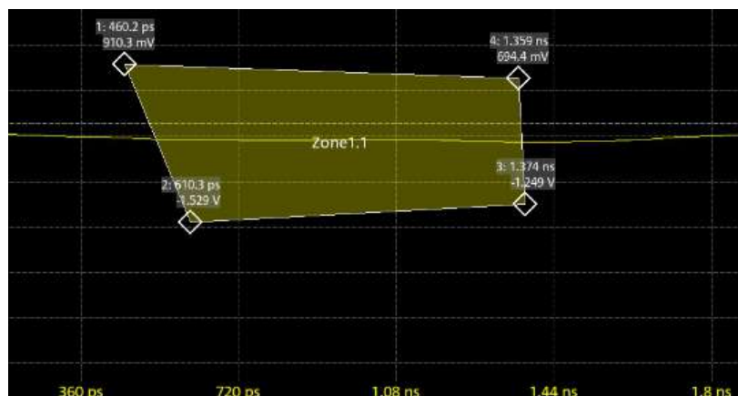
Figure 7-11: 1 area of a trigger zone
