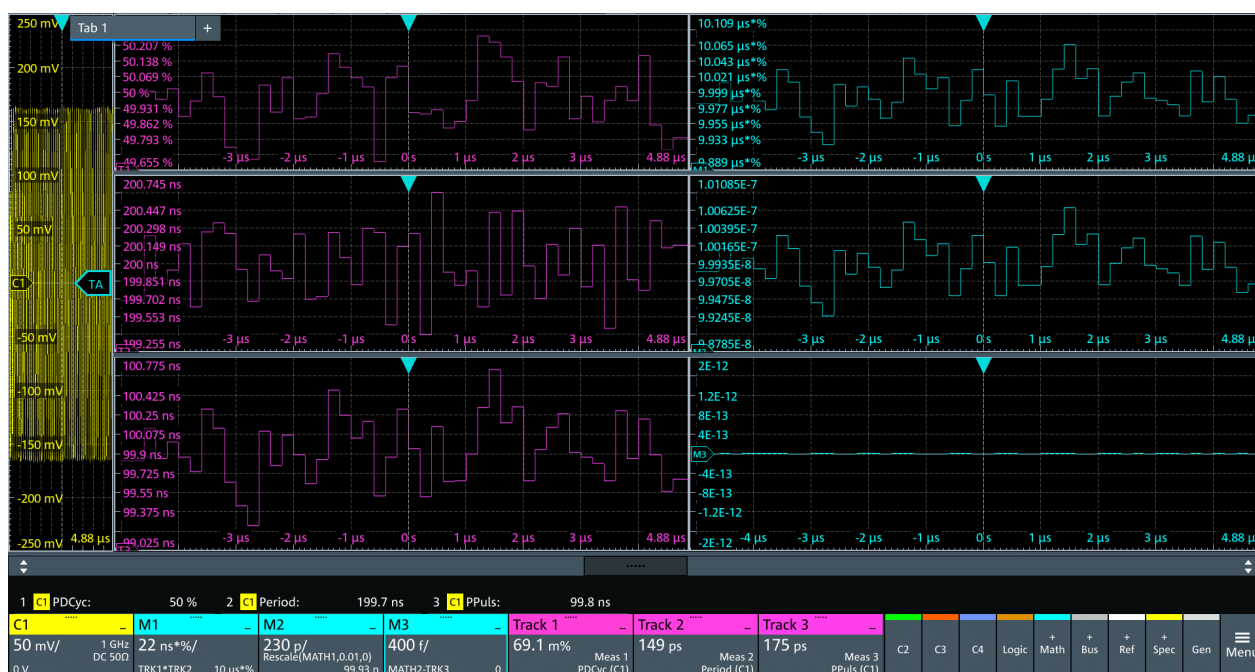
Figure 9-7: Tracks used in math functions
